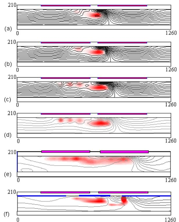
**Figure 1. Striation phenomena appearing in the PDP cell by kinetic and fluid simulations**
