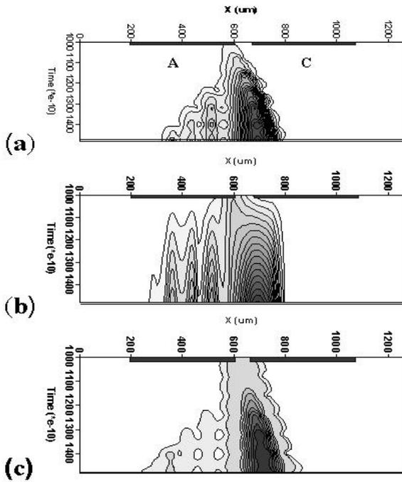
**Figure 2. The discharge propagation of (a) electron (b)  $Xe^+$  and (c)  $Ne^+$ .**
