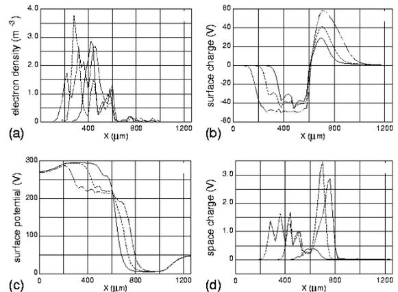
**Figure 4. (a) Electrons on the dielectric surface, (b) total surface charge on the front dielectric material, (c) potential on the dielectric surface, and (d) space charge below 20 $\mu m$  from the dielectric surface.**
