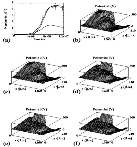
**Figure 3. (a) The number trace and (b)-(f) potential changes in the PDP cell with time (the arrows indicate the time of (b) – (f)).**
