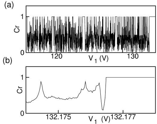
Fig. 7. (a) Correlation values for the mode transition diagram of Fig. 5. (b) Magnification of (a) near the transition from  $1P$  to Chaos.
