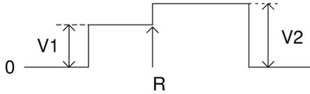
Fig. 1. Two-tiered pulse used in the simulation. The total pulse width is 5  $\mu$ s. The repetition frequency of the pulse is 0.125 MHz.  $V_1$  and  $V_2$  are the voltages of two tiers, and  $R$  is the beginning of the second tier.
