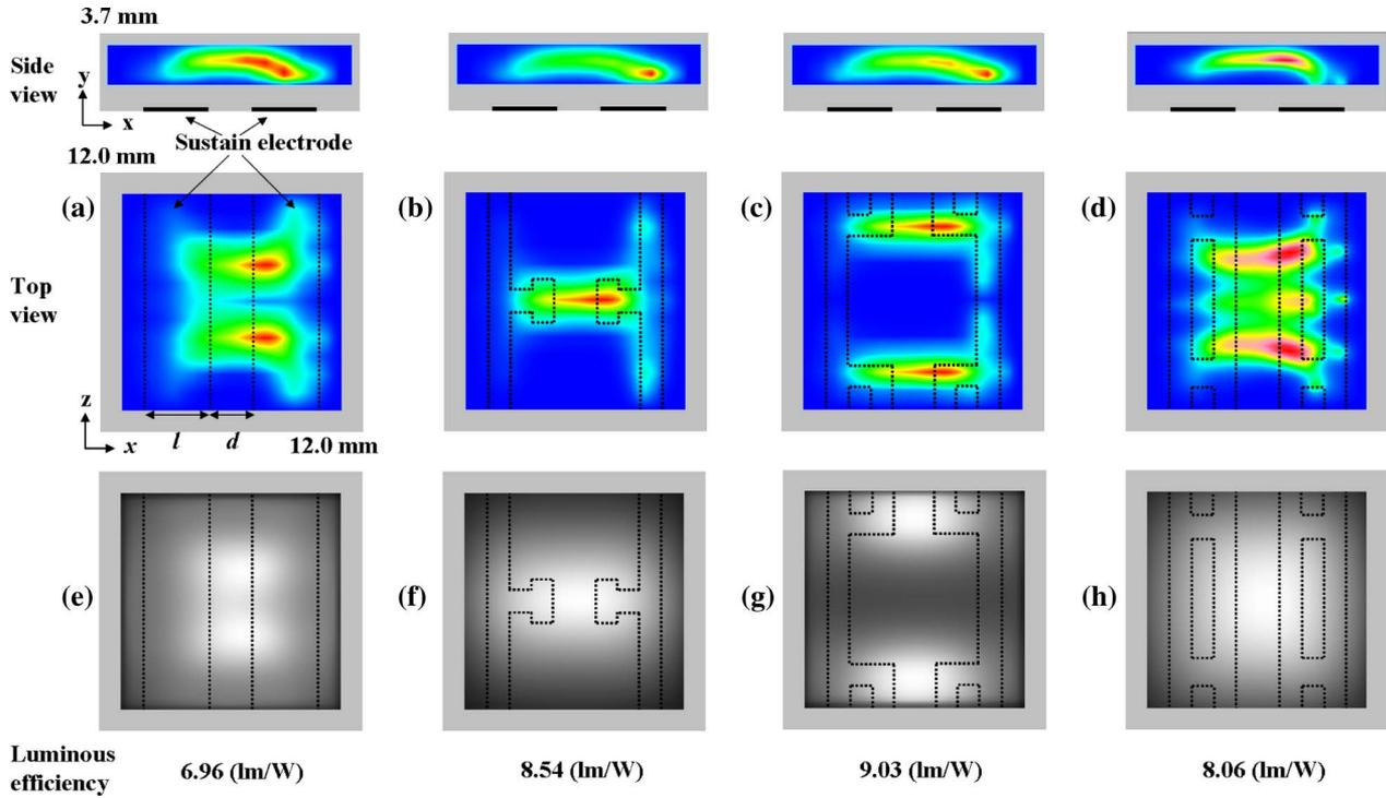
Fig. 1. Side- and top-views of  $Xe^*(^3P_1)$  density in (a) reference model, (b) T-, (c) Pi-, and (d) ladder-shape models, and the total light distribution in (e) reference model, (f) T-, (g) Pi-, and (h) ladder-shape models.
