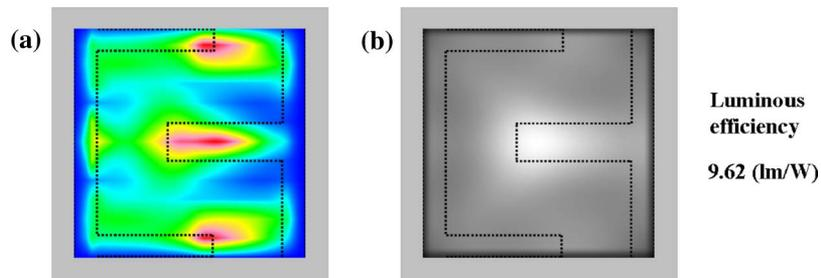
Fig. 2. (a)  $Xe^*(^3P_1)$  density profile and (b) total light distribution in the interlocked-shape model.
