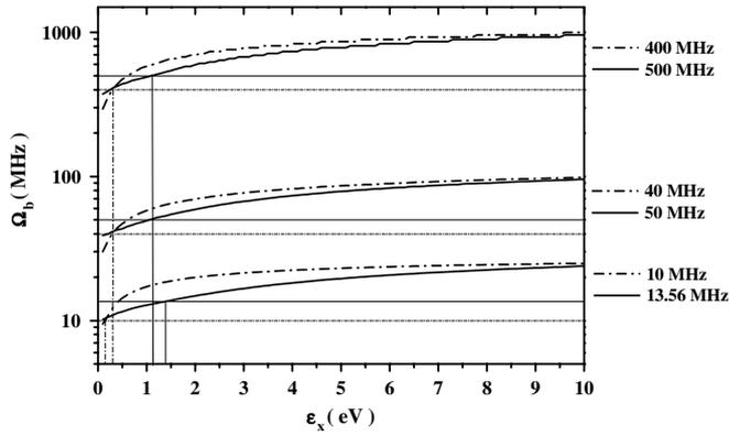
**Figure 2.** Electron bounce frequency as a function of the  $x$ -directional energy for capacitively coupled discharges driven by a 40 V voltage source in three regimes (1 mm, 1 cm and 4 cm). The horizontal straight lines indicate the driving frequencies.
