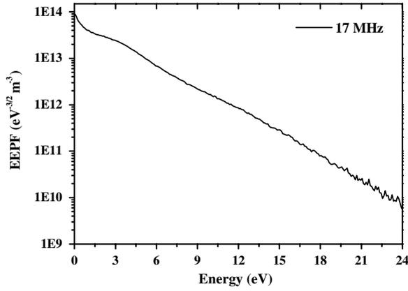
**Figure 4.** EEPF at the centre of the discharge for a capacitively coupled discharge driven by 17 MHz with a 40 V voltage source at 25 mTorr.
