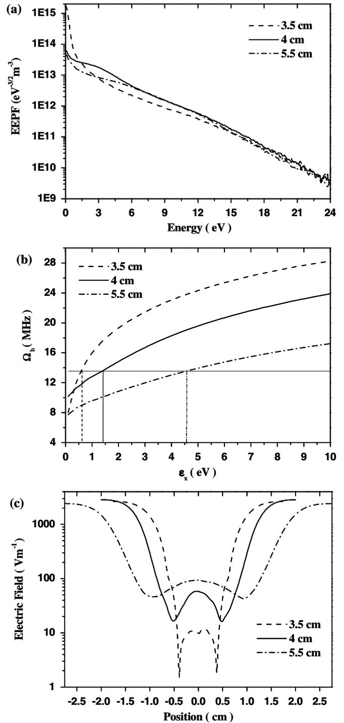
**Figure 3.** Simulation results for three capacitively coupled discharges driven at 13.56 MHz: (a) EEPFs at the centre of the discharge, (b) electron bounce frequency as a function of the  $x$ -directional energy and (c) the spatial profiles of the rf electric field (the centre of the discharge is set to zero for a comparison of the profiles for different gap distances).
