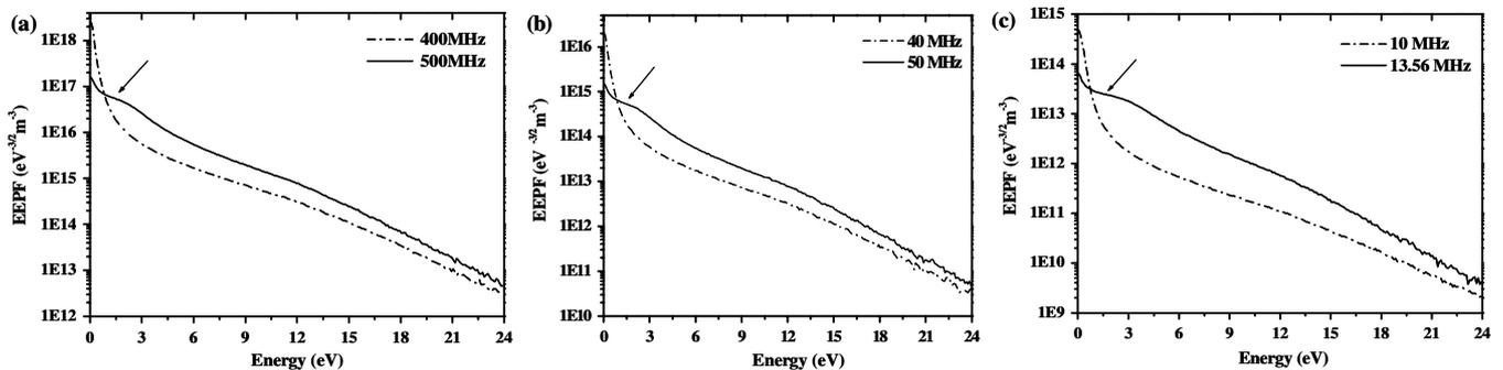
**Figure 1.** EPPFs at the centre of the discharge for capacitively coupled discharges driven by a 40 V voltage source in three regimes: (a) 1 mm (1 Torr), (b) 1 cm (100 mTorr) and (c) 4 cm (25 mTorr).
