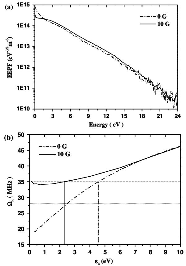
**Figure 5.** Simulation results for two capacitively coupled discharges driven at 35 MHz: (a) EEPFs at the centre of the discharge and (b) electron bounce frequency as a function of the  $x$ -directional energy (the dashed and the dotted lines indicate the driving frequency ( $\sim 35$  MHz) and the cyclotron frequency ( $\sim 28$  MHz), respectively).
