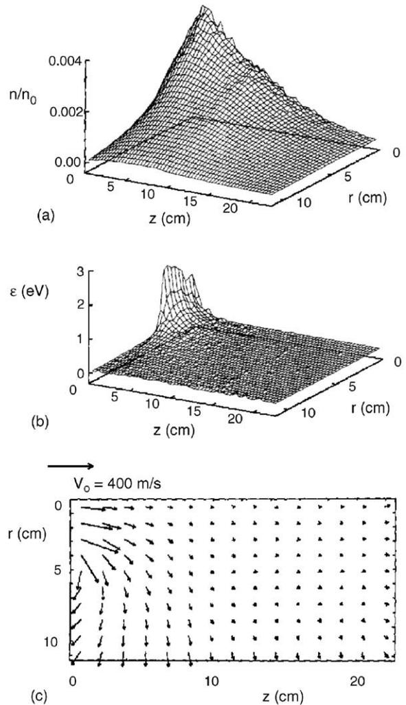
Fig. 7. Steady-state behavior of sputtered Cu atoms in a DSMC simulation: (a) density  $n$ ; (b) mean kinetic energy per particle,  $\epsilon$ ; (c) velocity fluid  $u$  (from [24]).
