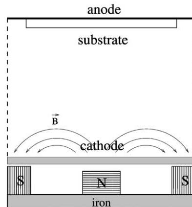
Fig. 1. Schematic diagram of typical magnetron sputtering system.
