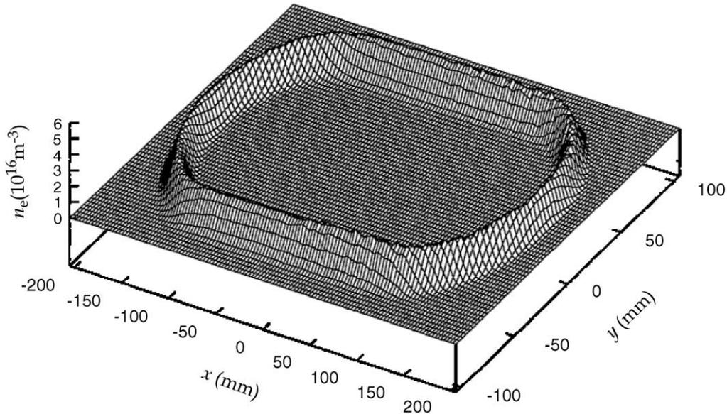
Fig. 3. Number densities of electrons in the  $xy$ -plane.  $z$ -direction is from cathode to substrate (from [8]).
