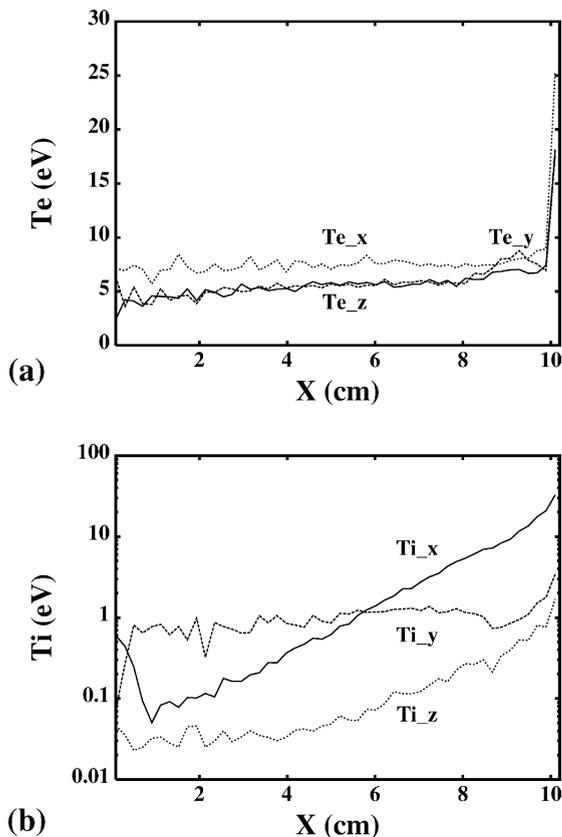
Fig. 11. Spatial temperature distributions of (a) electrons and (b) ions (from [34]).
