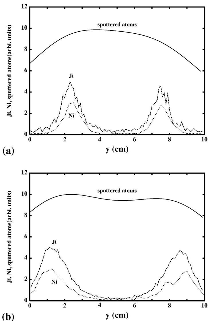
Fig. 8. Deposition profiles dependent on different magnetic field distributions (from [34]).
