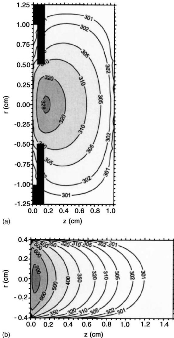
Fig. 9. 2D background gas temperature profile. The cathode is found at the left end of both figures, whereas the other boundaries represent the anodes (from [28]).
