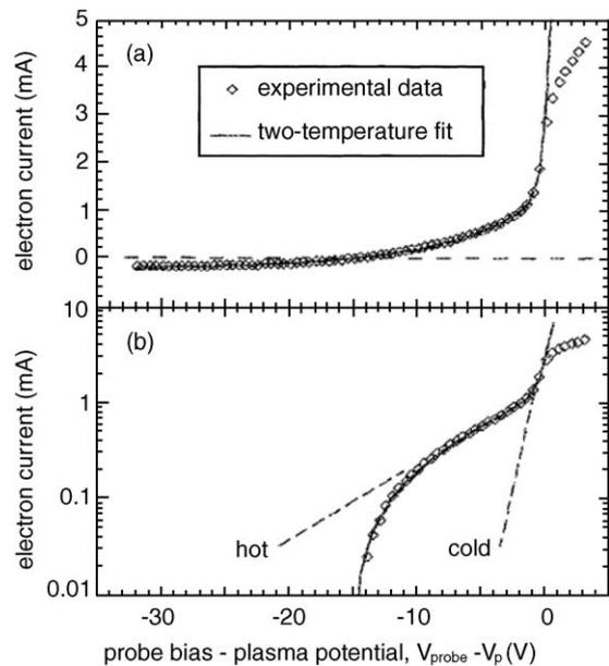
Fig. 10. Two-temperature probe characteristics in: (a) the electron current with two-temperature fitting; (b) log scale of electron current that shows two slopes (from [40]).
