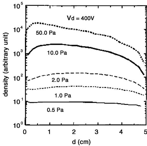
Fig. 6. The density profiles of sputtered atoms at various pressures (from [25]).  $d$  is cathode–substrate separation and discharge voltage is 400 V.
