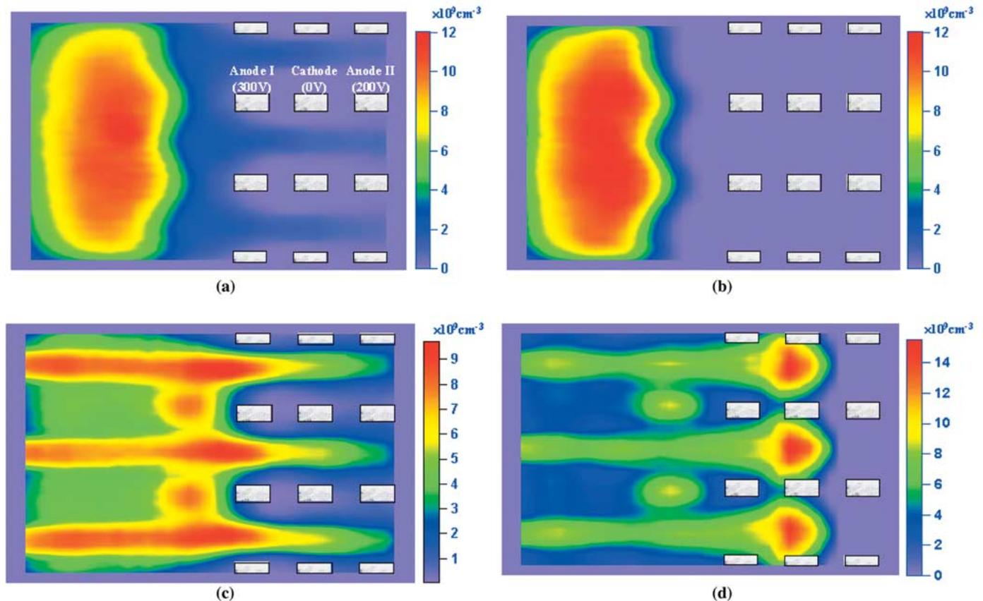
Fig. 1. Snapshot of a particle density distribution by PIC simulation. (a) Ion and (b) electron density distributions in the conventional ion gun. (c) Ion and (d) electron density distributions in the ion gun with the electron beam of 1000 eV and the magnetic field of 100 G. Magnetic field is perpendicular to the electron beam.
