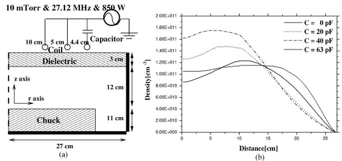
Fig. 1. (a) Schematic diagram; (b) radial distribution of plasma density with respect to the capacitor.
