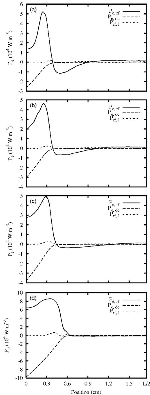
FIG. 1. Power deposition profiles at (a) 100, (b) 80, (c) 60, and (d) 40 MHz. Only the left-hand side of the system is plotted.
