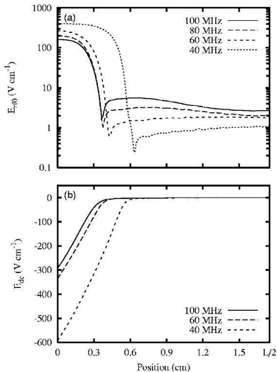
FIG. 2. The spatial profiles of (a) the rf electric field and (b) the dc electric field for different frequencies. Only the left-hand side of the system is plotted.
