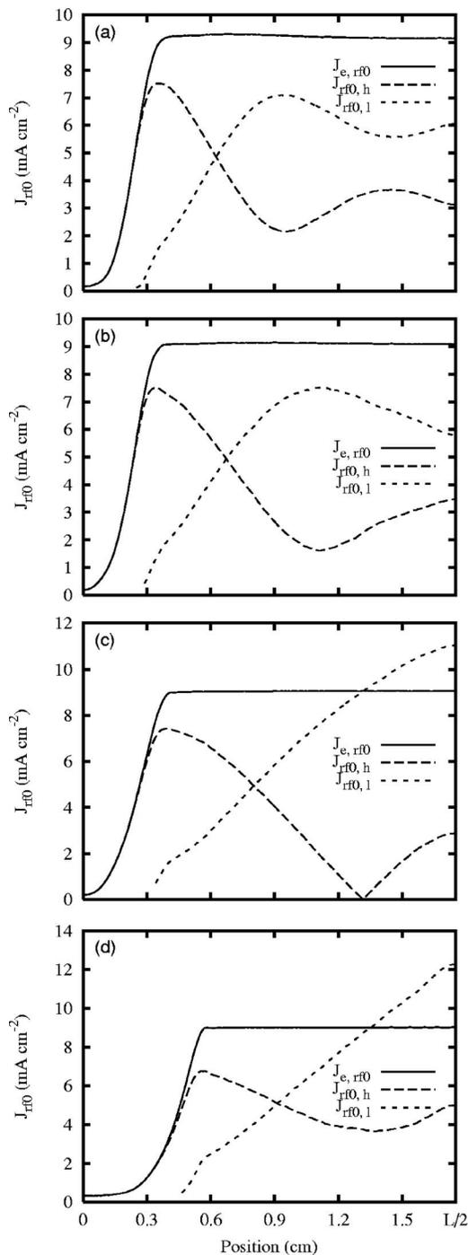
FIG. 3. The spatial profiles of the rf electron currents at (a) 100, (b) 80, (c) 60, and (d) 40 MHz. Only the left-hand side of the system is plotted.
