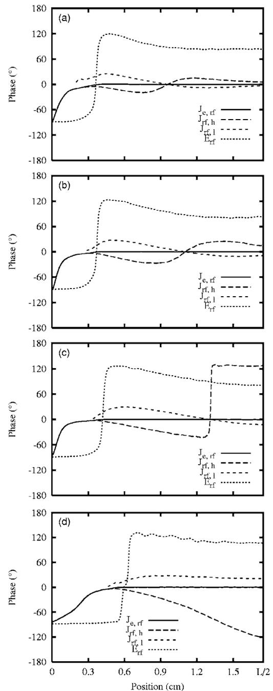
FIG. 4. The spatial profiles of the phase of the rf electric field and the rf electron currents at (a) 100, (b) 80, (c) 60, and (d) 40 MHz. They are calculated with respect to the phase of the applied current. Only the left-hand side of the system is plotted.
