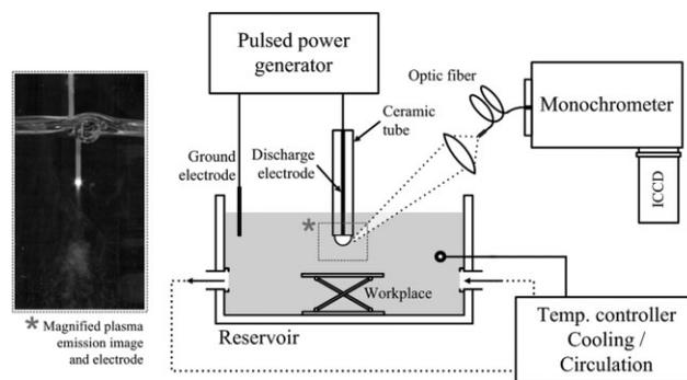
**Figure 1.** A schematic diagram of the pin electrode saline plasma system configuration for the feasibility studies of intravascular blood clot removal.
