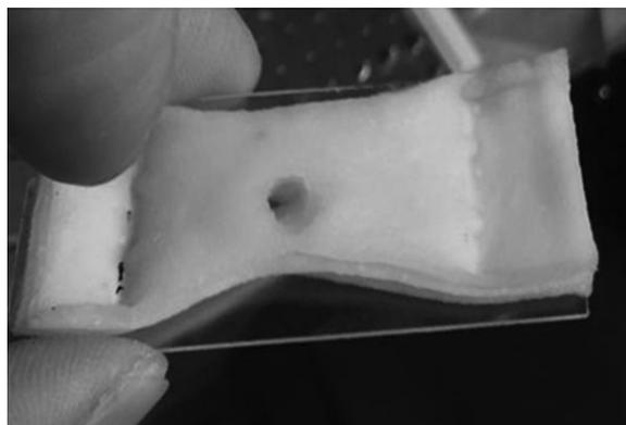
**Figure 2.** Each collagen sheet is soaked with soft horse blood and a stack of eight such sheets was used as a proxy model of a chronic total occlusion blood clot. Point source electrode driven saline plasma radicals totally etched through all eight layers, removing a 2  $\text{mm}^3$  volume per minute.
