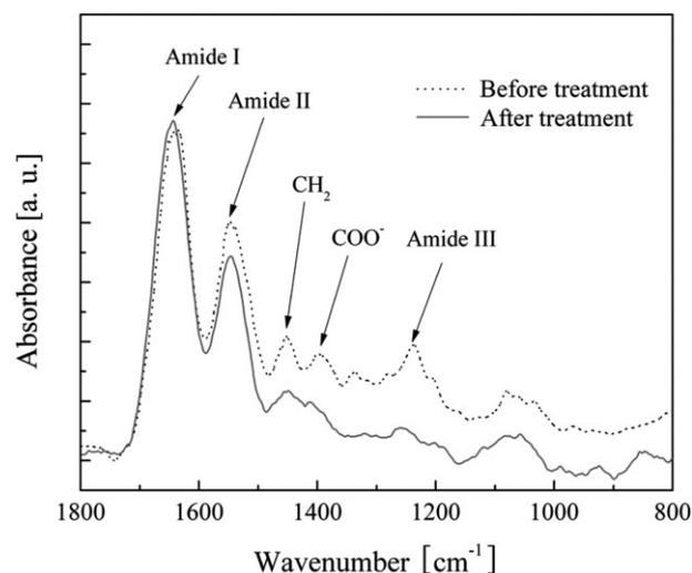
**Figure 5.** FT-IR spectra analysis for the collagen sheets treated in saline plasma as compared to untreated samples, in the wavelength region from 1800 to 800  $\text{cm}^{-1}$ .
