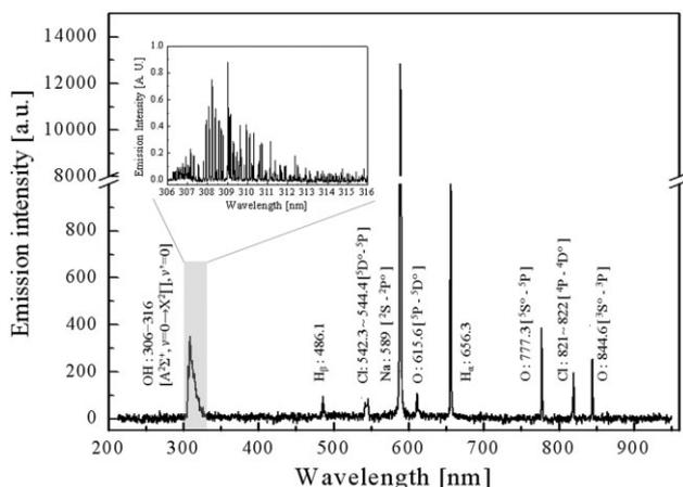
**Figure 4.** The dominant spectral lines emitted by the saline plasma. Note the presence of two Cl emissions under our experimental saline plasma conditions, indicating the conversion of the negative Cl ion to neutral chlorine in our conditions.
