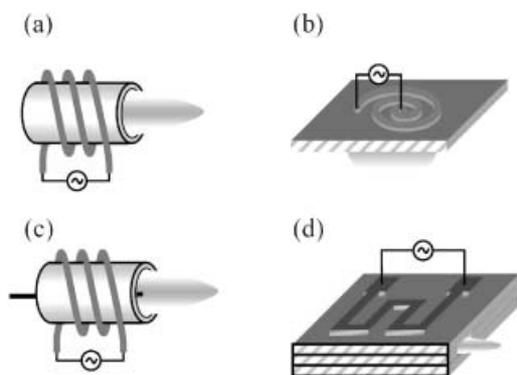
**Figure 4.** Schematics of inductively coupled microplasma sources: a) coil,<sup>[134]</sup> b) planar spiral,<sup>[134]</sup> c) coil + filament,<sup>[135]</sup> and d) serpentine.<sup>[136]</sup>
