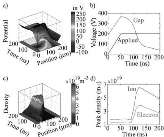
**Figure 12.** Potential and density profiles in a Ne/Xe(5%) DBD microdischarge at 300 Torr (40 kPa). a) Time evolution of the potential profile. b) Applied voltage and gap voltage as a function of time. c) Time evolution of the electron density profile. d) Maximum electron and ion densities as a function of time. The discharge is operated at 200 V/150 kHz and the results presented account for residual charges on the dielectrics from previous pulses.
