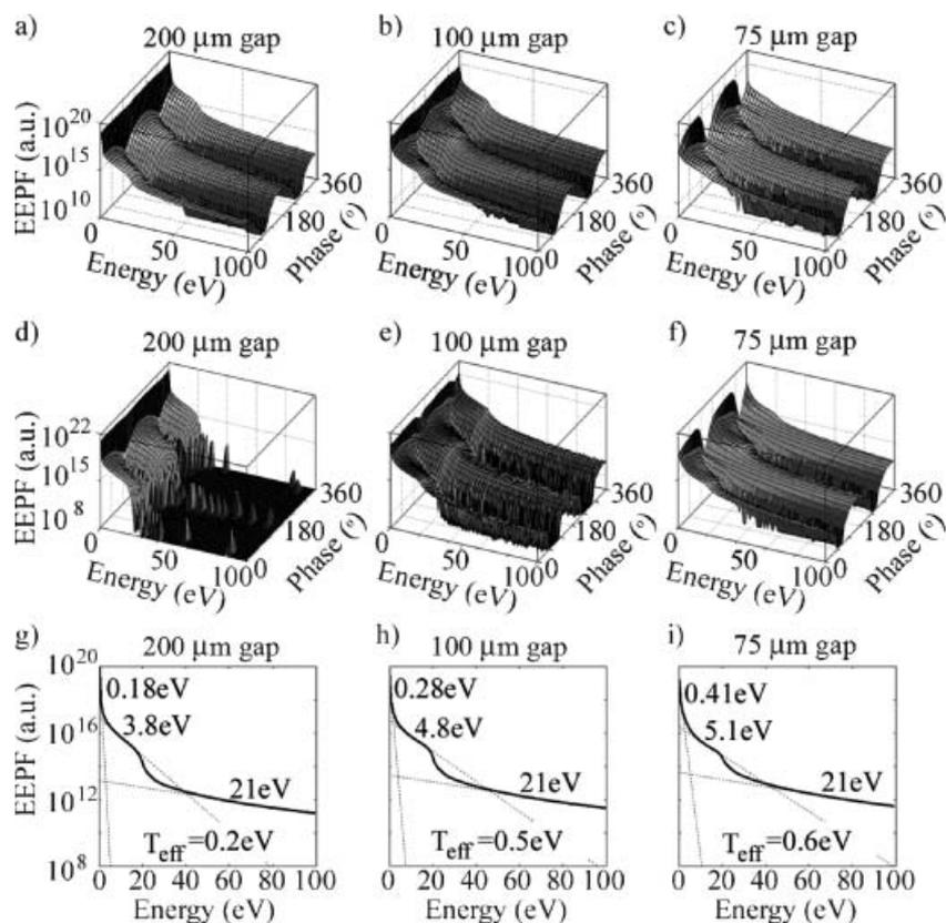
**Figure 9.** Time evolution of the EEPF in three atmospheric-pressure He microplasmas driven at  $1 \text{ A} \cdot \text{cm}^{-2}$ . a–c) Space-averaged EEPF. d–f) EEPF in the centre of the discharge. g–i) Space- and time-averaged EEPF. Figure reprinted with permission from ref.<sup>[165]</sup>. Copyright 2007 American Physical Society.
