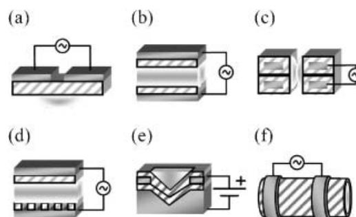
**Figure 2.** Schematics of dielectric barrier microdischarges: a) coplanar DBD,<sup>[16]</sup> b) parallel plate DBD,<sup>[91]</sup> c) coaxial DBD,<sup>[92]</sup> d) capillary plasma electrode discharge,<sup>[14]</sup> e) pyramidal DBD,<sup>[89]</sup> and f) capillary discharge/plasma pencil/plasma jet.<sup>[93]</sup> The solid colour represents metal electrodes and hatched objects represent dielectric materials.
