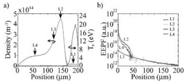
**Figure 7.** He DC microdischarge at atmospheric pressure.<sup>[177]</sup> a) Density and effective electron temperature profiles. b) EEPF at the four locations marked in (a). (Reprinted with permission, © 2007 IEEE.)
