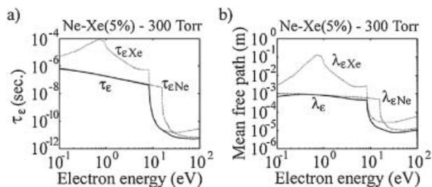
**Figure 14.** Electron energy relaxation time (a) and mean free path (b) in a 300 Torr (40 kPa) Ne/Xe(5%) mixture.
