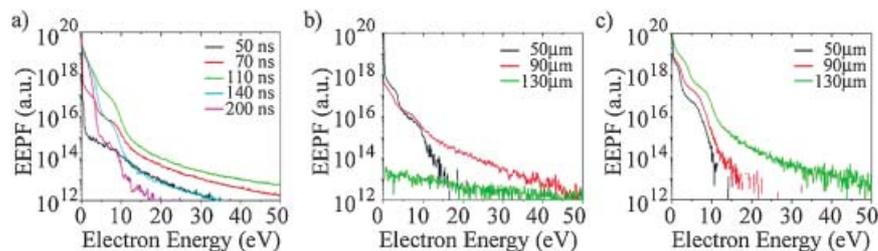
**Figure 13.** a) Time evolution of the EEPF in a Ne/Xe(5%) DBD discharge. EEPF at various locations measured at b)  $t = 70$  ns and c)  $t = 110$  ns. The distances are measured from the left hand side electrode (temporary anode).
