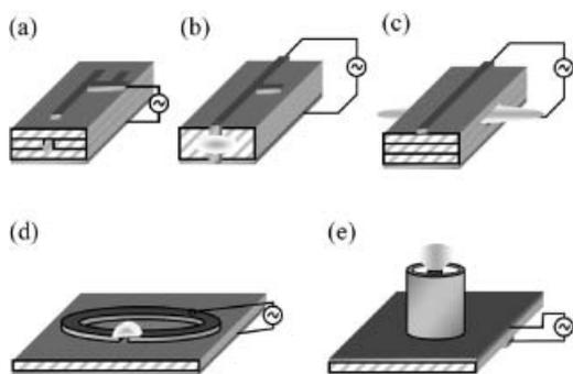
**Figure 5.** Schematics of microwave microplasma sources: a) microstrip linear resonator,<sup>[141–143]</sup> b) microstrip linear resonator with engineered end,<sup>[144]</sup> c) surface wave launcher based on microstrip technology,<sup>[144]</sup> d)  $\lambda/2$  microstrip split-ring resonator,<sup>[61,63,144,145]</sup> and e) coaxial source.<sup>[51,52,149,150]</sup>
