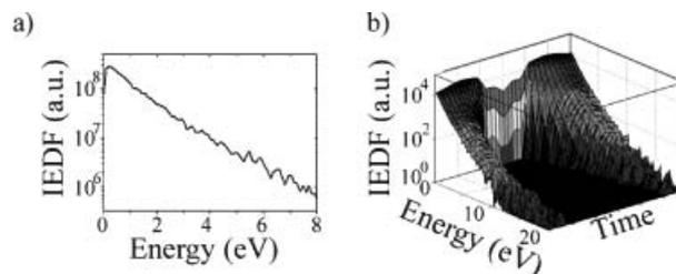
**Figure 15.** Energy distribution function of  $\text{He}^+$  ions impinging on the electrode of a) 200  $\mu\text{m}$  DC, and b) 100  $\mu\text{m}$  RF microdischarges at atmospheric pressure. The average ion energy is  $T_i = 1\text{--}3$  eV.
