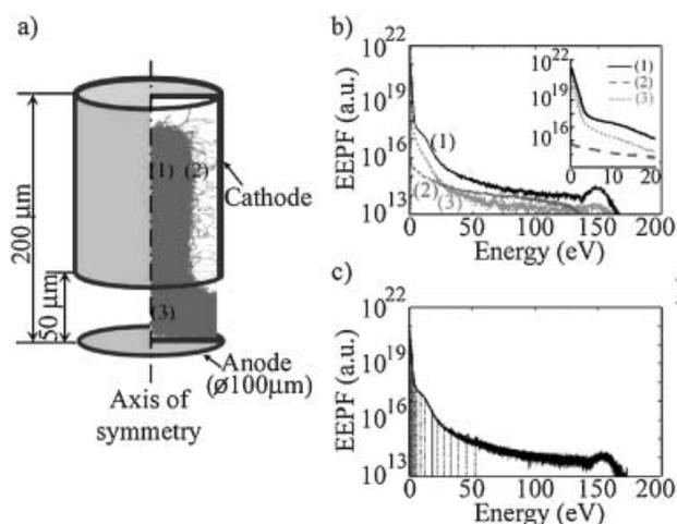
**Figure 8.** Microhollow cathode discharge in Ar at 10 Torr (1.3 kPa). a) Trajectories of electrons showing the pendular motion of the electrons.<sup>[82]</sup> b) EPPF vs. kinetic energy at various locations showing the high energy tail created by pendular electrons.<sup>[82]</sup> c) EPPF vs. total energy at various locations.
