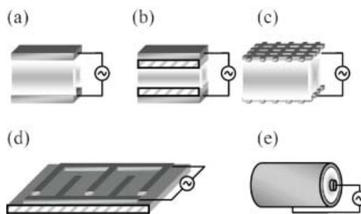
**Figure 3.** Schematics of RF capacitively coupled microplasmas: a) parallel plate with bare electrodes,<sup>[123]</sup> b) parallel plate with dielectric-covered electrodes,<sup>[124]</sup> c) grid electrodes,<sup>[125]</sup> d) comb electrodes,<sup>[126]</sup> and e) coaxial jet.<sup>[127]</sup>
