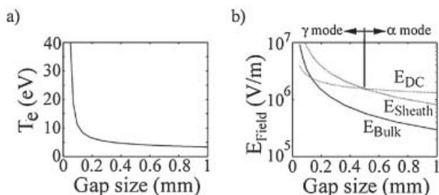
**Figure 11.** Global model of an atmospheric-pressure Helium plasma driven at 13.56 MHz with  $n_e = 10^{11} \text{ cm}^{-3}$ . a) Electron temperature and b) electric field in the bulk and in the sheath as a function of the gap size.  $E_{DC}$  in (b) is the DC breakdown electric field for helium at atmospheric pressure [1] assuming  $\gamma = 0.1$ .
