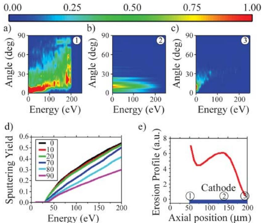
**Figure 18.** Erosion profile in a microhollow cathode discharge. a–c) Energy and angle distribution of ions impinging onto the three different regions of the cathode shown in (e). d) Sputtering yield of Mo by Ar<sup>+</sup> ions. e) Erosion profile. The incidence angle is measured with respect to the cathode surface normal, i.e., an ion impinging perpendicularly to the surface has an incidence angle of 0 degrees.
