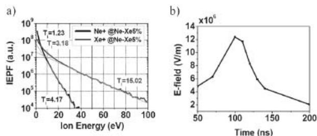
**Figure 16.** a) Time-integrated ion energy probability function of  $\text{Ne}^+$  and  $\text{Xe}^+$  ions impinging on the dielectric surface. b) Evolution of electric field in the cathode sheath for a 300 Torr Ne/Xe(5%) DBD discharge.
