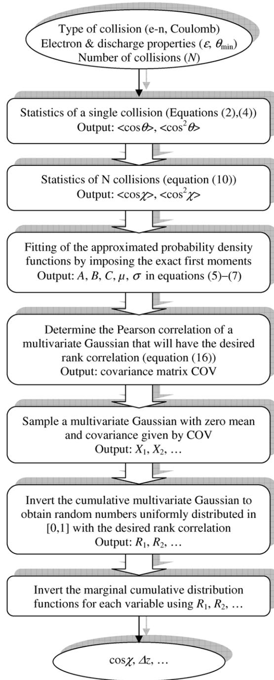
**Figure 8.** Flow diagram for computing the scattering angle and the net displacement of a particle undergoing multiple collisions. Correlation between the angle and displacement is enforced by a Gaussian copula.
