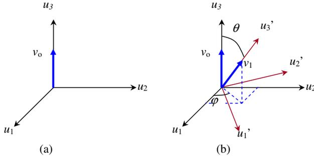
**Figure 2.** Coordinate system rotation following the scattering of the velocity vector after a single collision. (a) Before and (b) after the collision.
