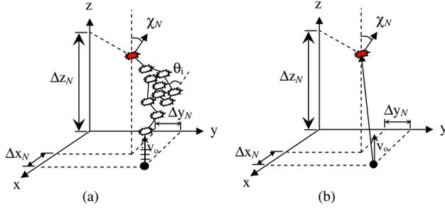
**Figure 1.** Advancing of a particle undergoing multiple collisions. (a) PIC-MCC approach in which  $v\Delta t \ll 1$ : each collision is modelled individually and several time steps are simulated in between collisions. (b) PIC-MCC approach in which  $v\Delta t \gg 1$ : the particle is directly positioned at the final position after  $N$  collisions and only the net displacement ( $\Delta x_N$ ,  $\Delta y_N$ ,  $\Delta z_N$ ) and the cumulative scattering angle ( $\chi_N$ ) are computed.
