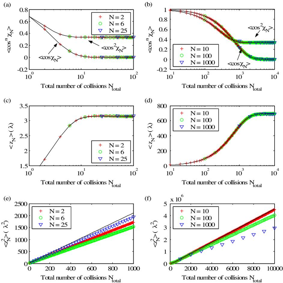
**Figure 6.** Comparison of the first moments of (a), (b) the scattering angle and (c)–(f) the particle position for various values of  $N$  (number of collisions modelled in one iteration). Symbols represent PIC simulation results for (a), (c), (e) electron-neutral collisions (500 eV electrons) and (b), (d), (f) Coulomb collisions ( $\theta_{\min} = 1^\circ$ ). The black solid lines represent the theoretical values (equations (10) and (12)).
