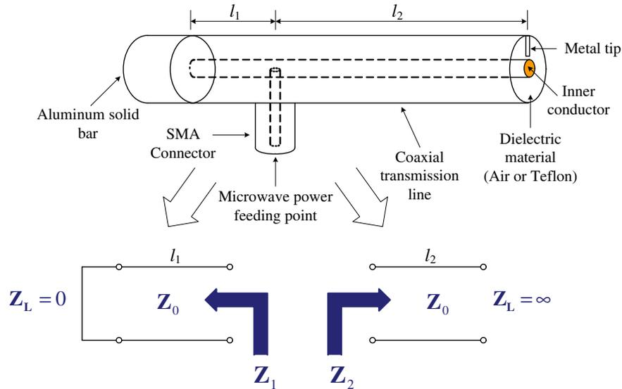
**Figure 1.** The schematic of the CTLR and the simplified microwave model.
