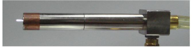
**Figure 7.** Argon microplasma jet of device II with 2.5 W input power and 2 slm flow rate at atmospheric pressure.
