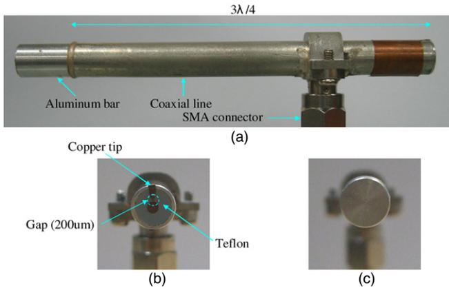
**Figure 2.** Device I: CTLR for operation at  $\sim 2.45$  GHz. (a) Side, (b) front and (c) rear view.
