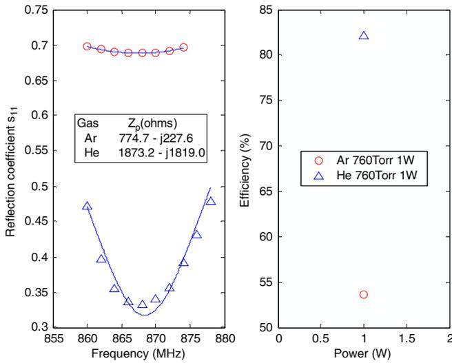
**Figure 8.** Plasma impedance and power efficiency of argon and helium microplasmas at atmospheric pressure with device II.
