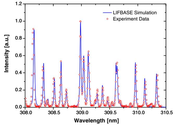
**Figure 9.** The rotational temperature estimation (400 K) of device II at 1.5 W input power and 15 slm gas flow rate at atmospheric pressure of the OH band based on LIFBASE.
