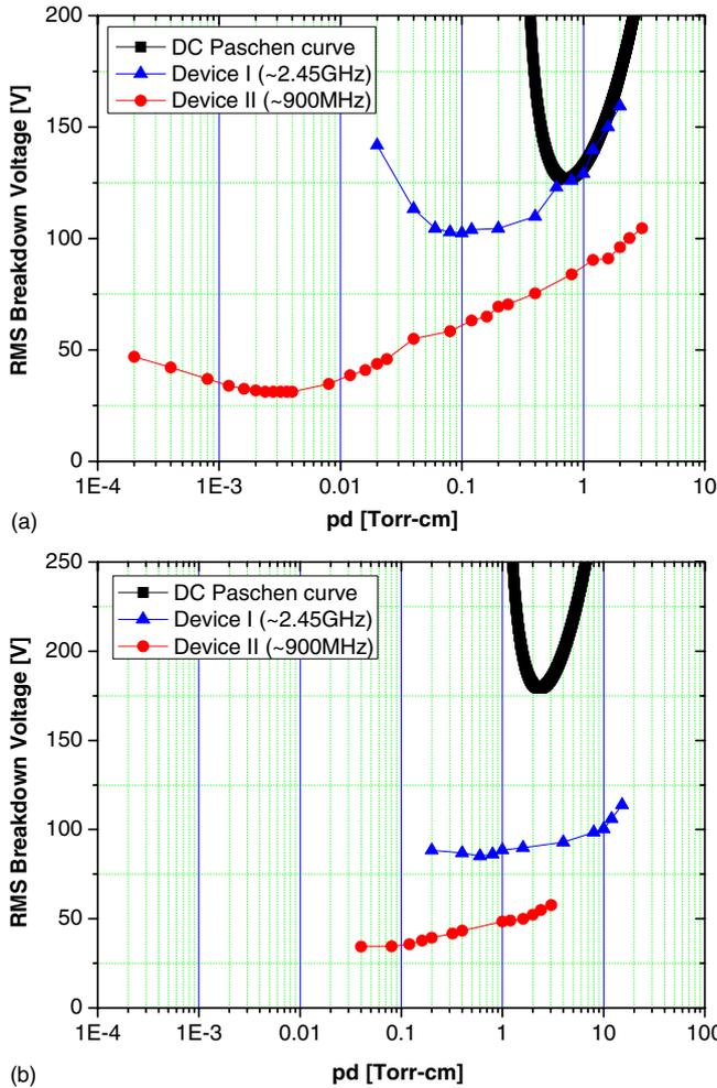
**Figure 5.** Comparison between theoretical dc Paschen curve and the microwave breakdown voltage of devices I and II. (a) Argon and (b) helium.
