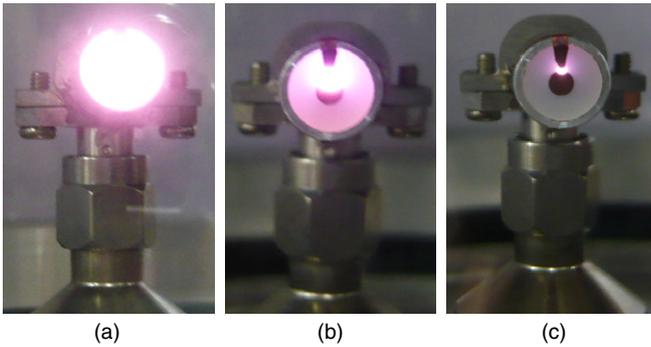
**Figure 6.** Helium microplasmas sustained with 0.3 W of device I: 10, 100 and 760 Torr (from (a) to (c)).
