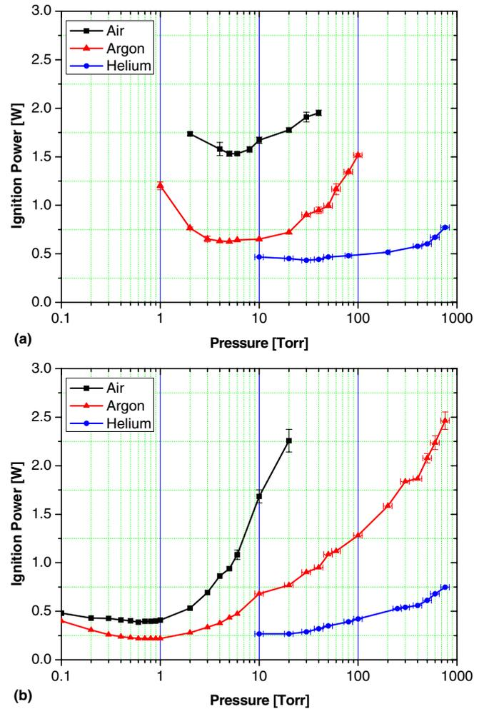
**Figure 4.** Ignition power in air, argon and helium of two devices: (a) device I ( $\sim 2.45$  GHz) and (b) device II ( $\sim 900$  MHz).
