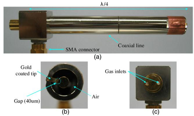
**Figure 3.** Device II: CTLR for operation at  $\sim 900$  MHz. (a) Side, (b) front and (c) rear view.
