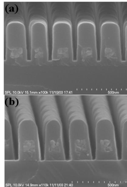
Fig. 5. No ARDE effect during the Si<sub>3</sub>N<sub>3</sub> spacer etching using a SF<sub>6</sub> neutral beam: (a) before spacer etching and (b) after spacer etching.
