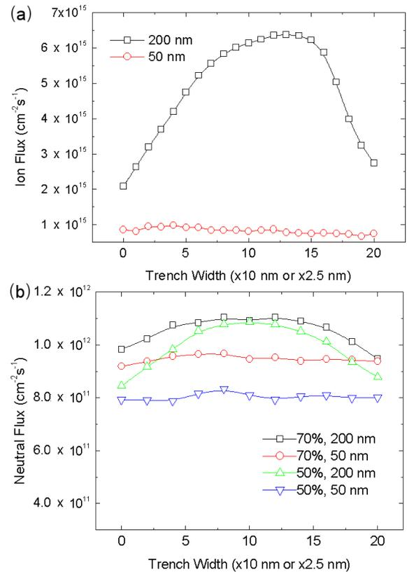
Fig. 3. (Variation of (a) the ion flux for RIE and (b) the neutral flux for the neutral beam arriving at the bottom of trench features having line widths of 200 nm and 50 nm and the initial aspect ratio of four. For the neutral beam, 50 % and 70 % of the directional angle ratio ([zero angle forward flux/total flux]  $\times 100$  %) were used for the neutral beam angle distribution arriving at the feature.
