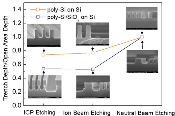
Fig. 4. The etch depth ratios between the open area ( $> 1.5\mu\text{m}$ ) and the trench area ( $400\text{ nm}$ ) of the photoresist-covered poly-Si on Si and the photoresist-covered poly-Si/SiO<sub>2</sub> on Si for an ICP, a reactive ion beam, and a neutral beam using SF<sub>6</sub>.
