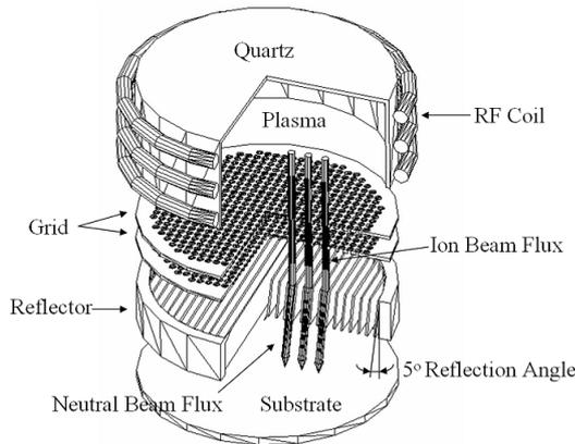
Fig. 2. Schematic diagram of the low-angle forward reflected neutral-beam system used in the experiment.
