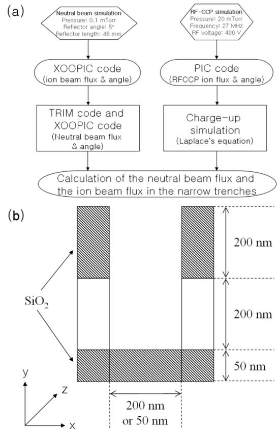
Fig. 1. (a) Flow chart of the flux simulation arriving at the trench bottom of a feature for the neutral beam etcher and for the rf CCP etcher. Figure 1(b) shows the shape of the trench feature used in the simulation.
