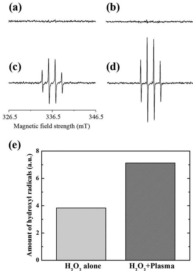
**Figure 5.** Typical ESR spectra measured from the mixture composed of H<sub>2</sub>O<sub>2</sub> (28%, 50  $\mu$ L) and DMPO (0.3 mol/L, 50  $\mu$ L) with (a, b) no additional reagent (group N) or (c, d) a piece of a tooth (group T): (a, c) before and (b, d) after plasma treatment for 1 minute. (e) Quantity of  $\cdot$ OH in group T before and after plasma treatment.
