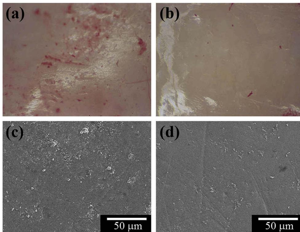
**Figure 4.** (a, b) Ponceau staining and (c, d) SEM images of the (a, c) control group ( $\text{H}_2\text{O}_2$  alone) and the (b, d) experimental group ( $\text{H}_2\text{O}_2$  plus plasma treatment).
