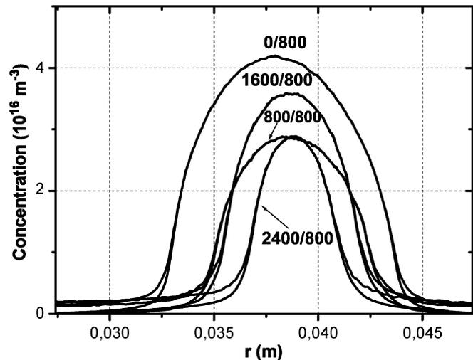
Fig. 6. Plasma density profiles for DF CCP. Conditions: 10/27 MHz; pressure 45 mtorr;  $V_{high} = 800$  V,  $V_{low}$  is varied.
