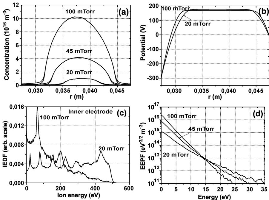
Fig. 2. Effect of pressure on (a) average plasma density; (b) average potential profiles; (c) IED at the powered (inner) electrode, and (d) EPPF. The IED spread corresponds to the mean potential drop at the inner electrode. Conditions: pressure 20, 45, and 100 mtorr,  $V_{rf} = 800$  V (amplitude), excitation frequency 27 MHz.
