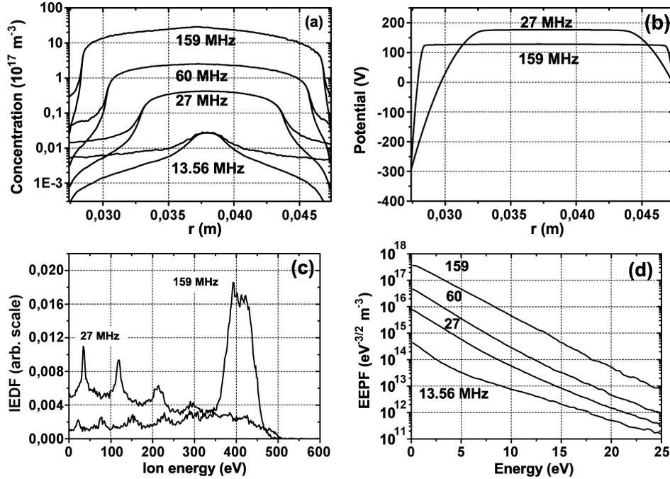
Fig. 4. Effect of frequency on (a) average plasma density; (b) average potential profile; (c) IED at the inner electrode, and (d) EPPF. The IED spread corresponds to the mean potential drop at the inner electrode. Conditions: pressure 45 mtorr,  $V_{rf} = 800$  V (amplitude), excitation frequencies 13.56, 27, 60, and 159 MHz.
