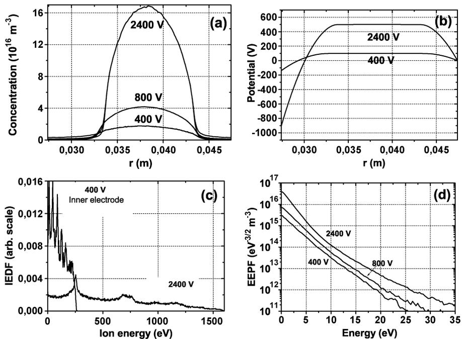
Fig. 3. Effect of applied voltage on (a) average plasma density; (b) average potential profiles; (c) IED at the inner electrode; and (d) EPPF. The IED spread corresponds to the mean potential drop at the inner electrode. Conditions: pressure 45 mtorr,  $V_{rf} = 400$ – $2400$  V (amplitude), excitation frequency 27 MHz.
