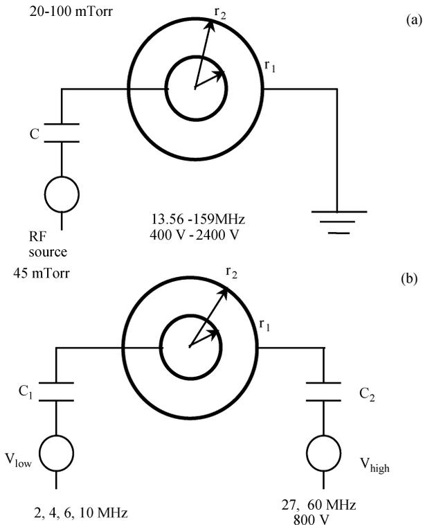
Fig. 1. Schematic diagram of the cylindrical (a) SF and (b) dual-frequency CCP sources.
