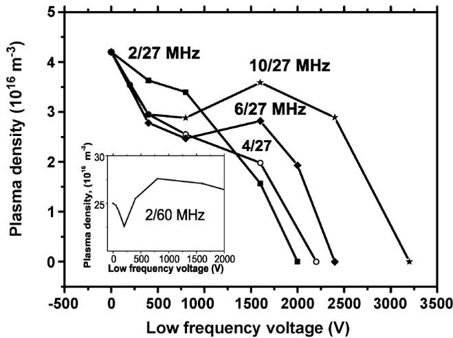
Fig. 7. Nonmonotonous behavior of plasma density versus low-frequency voltage for dual-frequency CCP. Conditions:  $X/27$  MHz,  $X = 2, 4, 6,$  and  $10$  MHz, pressure 45 mtorr,  $V_{\text{high}} = 800$  V,  $V_{\text{low}}$  is varied. The inset shows the similar effect for 2/60-MHz ratio.
