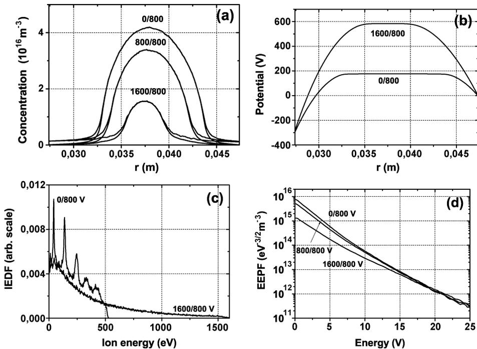
Fig. 5. Dual-frequency CCP (2/27 MHz). Effect of low-frequency voltage  $V_{low}$  on (a) average plasma density; (b) average potential profile; (c) IED at the inner electrode, and (d) EETF. The IED spread does not correspond to the mean potential drop at the inner electrode. Conditions: pressure 45 mtorr,  $V_{high} = 800$  V,  $V_{low}$  is varied.
