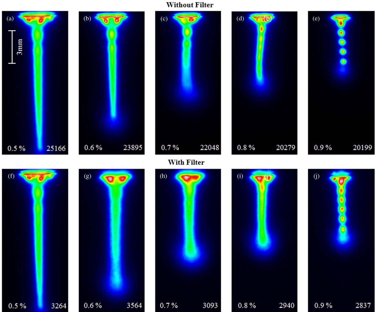
Fig. 2. ICCD image of microwave plasma plume with a variation of O<sub>2</sub> mixture (0.5 vol.% to 0.9 vol.%) with 4 W and 3 slm of argon gas flow. (a)–(e) Without filter. (f)–(j) With filter. Maximum intensity is presented at the right side of each image.
