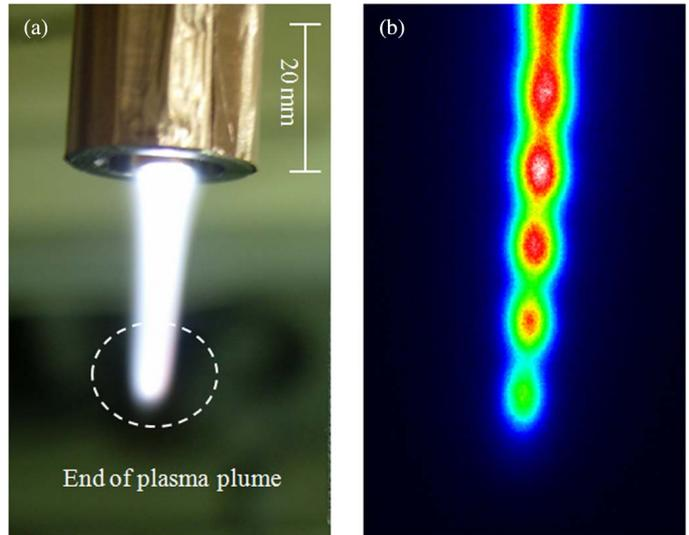
Fig. 1. 900-MHz microwave-induced plasma device. (a) Real plasma photograph with 3 W of effective power and 3 slm of argon gas flow rate. (b) ICCD image of end of plasma plume with the same condition.
