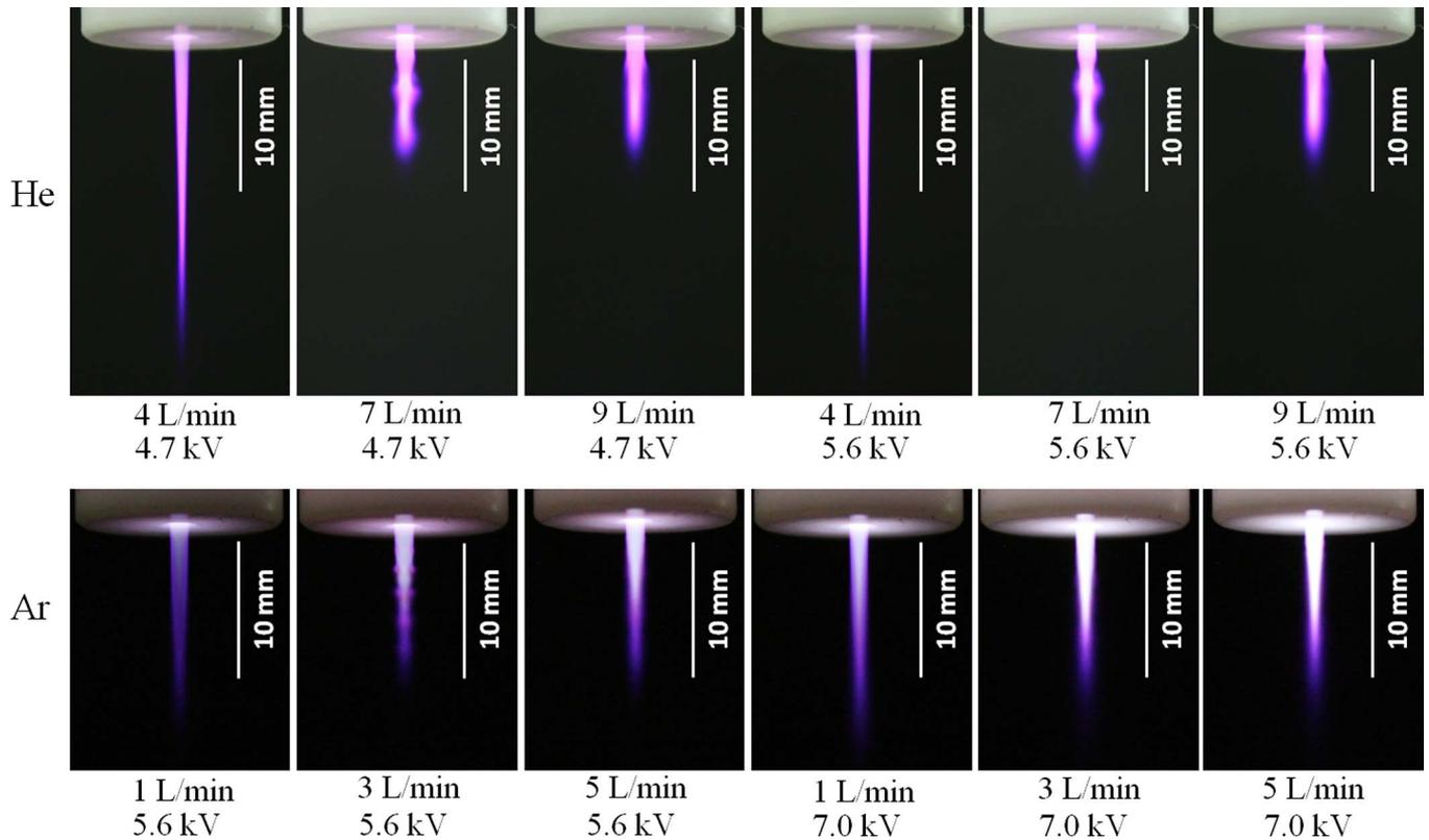
Fig. 1. Development of striated discharge patterns corresponding to the gas flow rate and driving voltage in He and Ar plasma jets. (The exposure time of the digital camera is 1 s for He plasma and 1/3 s for Ar plasma.)
