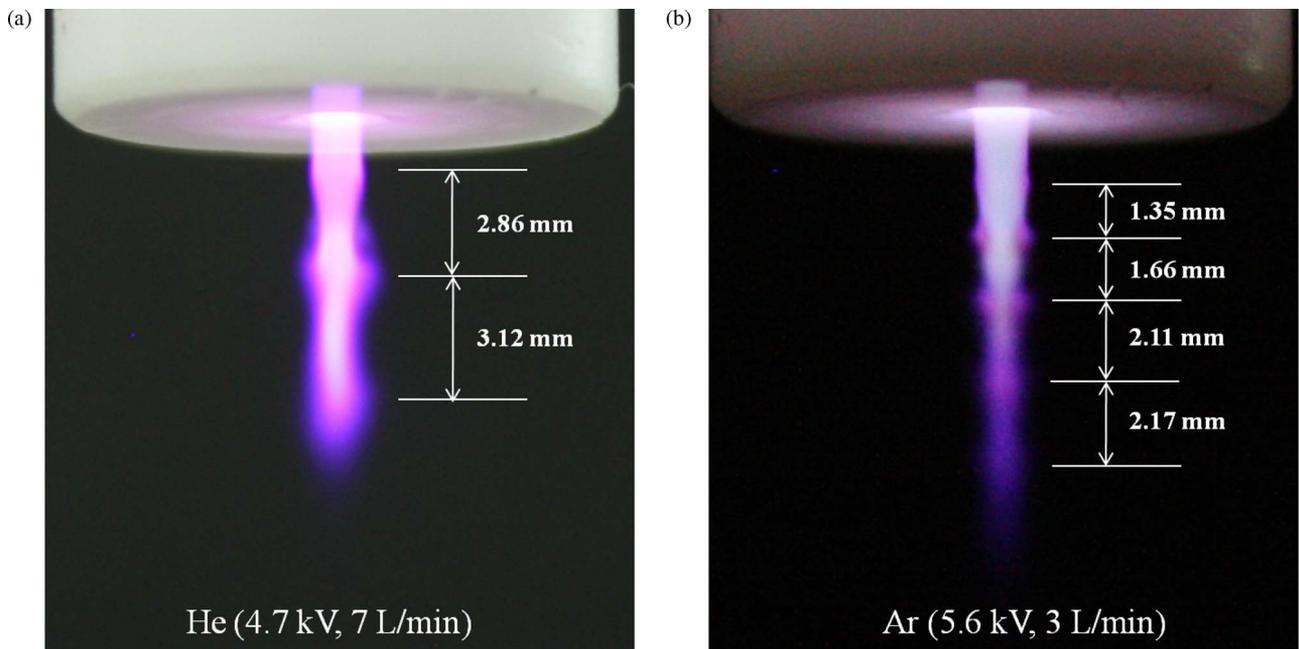
Fig. 2. Striated discharge patterns in (a) the He APPJ at 4.7 kV and 7 L/min and (b) the Ar APPJ at 5.6 kV and 3 L/min.
