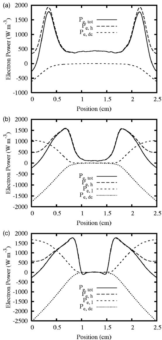
FIG. 3. Simulation result without SEE. The spatial profile of the power consumed by electrons for low-frequency currents of (a) 0, (b) 0.15, and (c) 0.2 mA cm<sup>-2</sup>.
