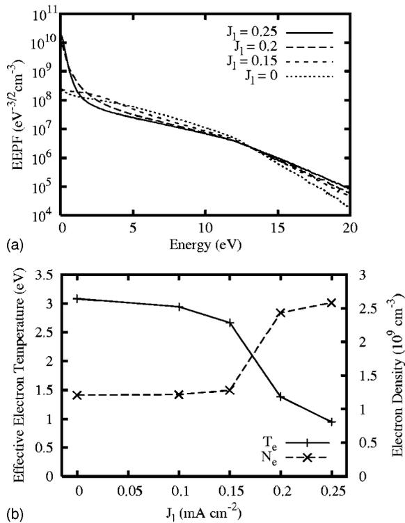
FIG. 1. Simulation result without SEE: (a) Electron energy probability functions at the discharge center for various low-frequency currents. (b) Effective electron temperature and electron density at the discharge center as a function of the low-frequency current. Time-averaged values were presented.
