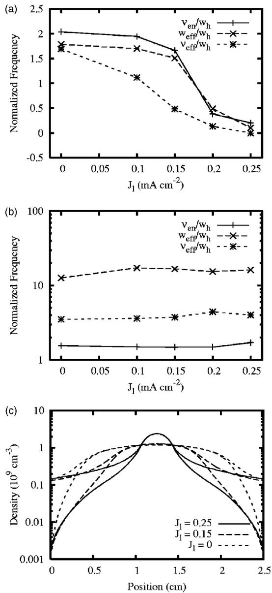
FIG. 5. Simulation result without SEE: Frequencies calculated at (a) the discharge center and (b) the position where the consumed power by electrons has the maximum value. (c) The spatial profiles of the ion and electron densities for low-frequency currents of 0, 0.15, and 0.25 mA cm<sup>-2</sup>.
