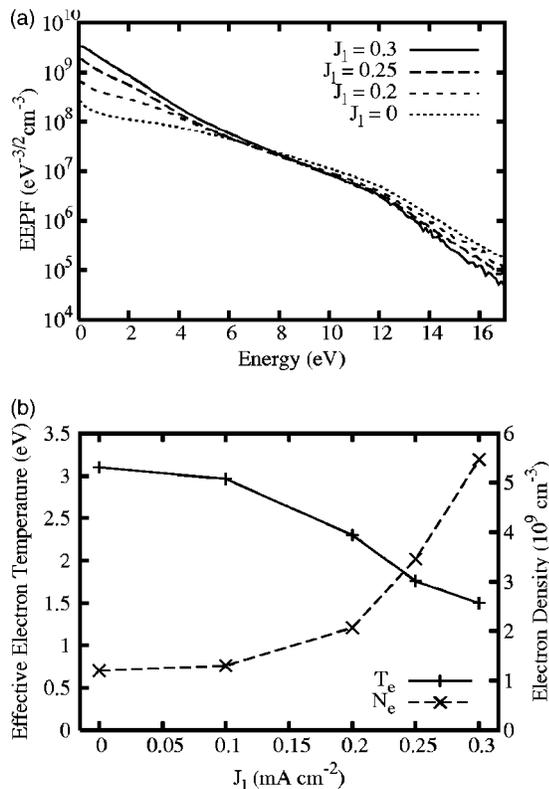
FIG. 9. Simulation result with SEE: (a) Electron energy probability functions at the discharge center for various low-frequency currents. (b) Effective electron temperature and electron density at the discharge center as a function of the low-frequency current.
