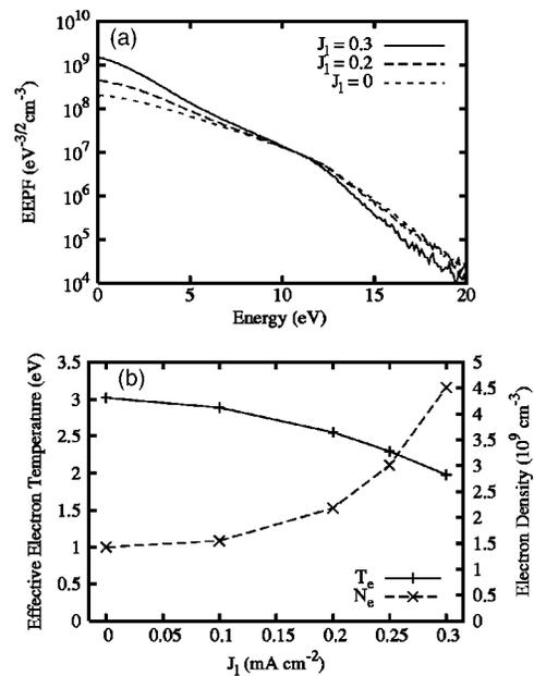
FIG. 12. Simulation result with SEE in the absence of the Ramsauer minimum: (a) Electron energy probability functions at the discharge center. (b) Effective electron temperature and electron density at the discharge center.
