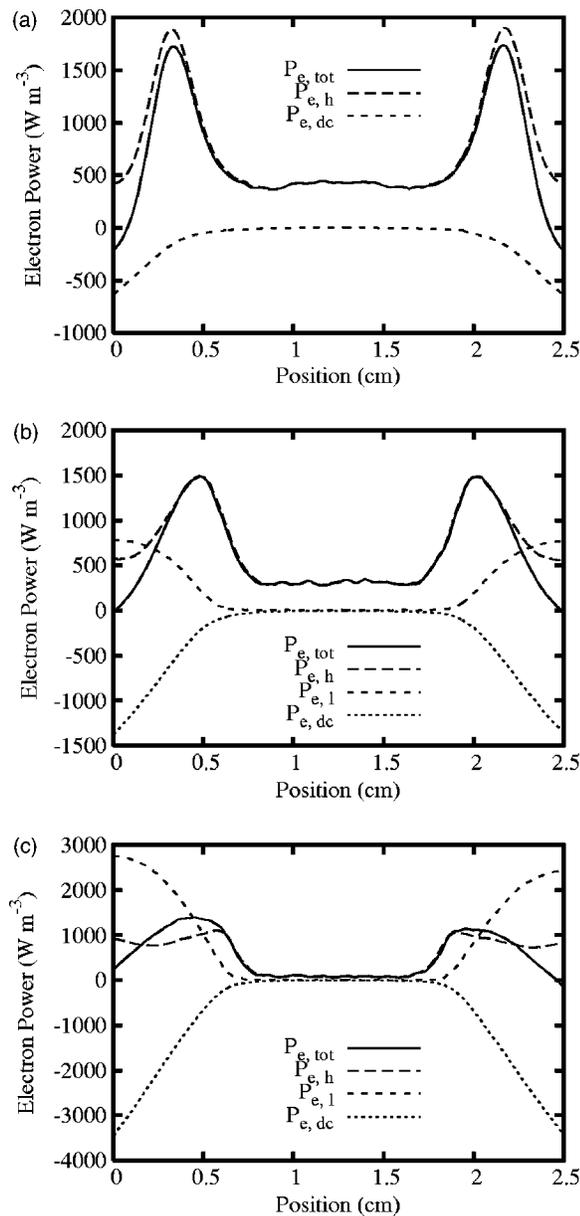
FIG. 11. Simulation result with SEE. The spatial profile of the power consumed by electrons for low-frequency currents of (a) 0, (b) 0.1, and (c) 0.2 mA cm<sup>-2</sup>.
