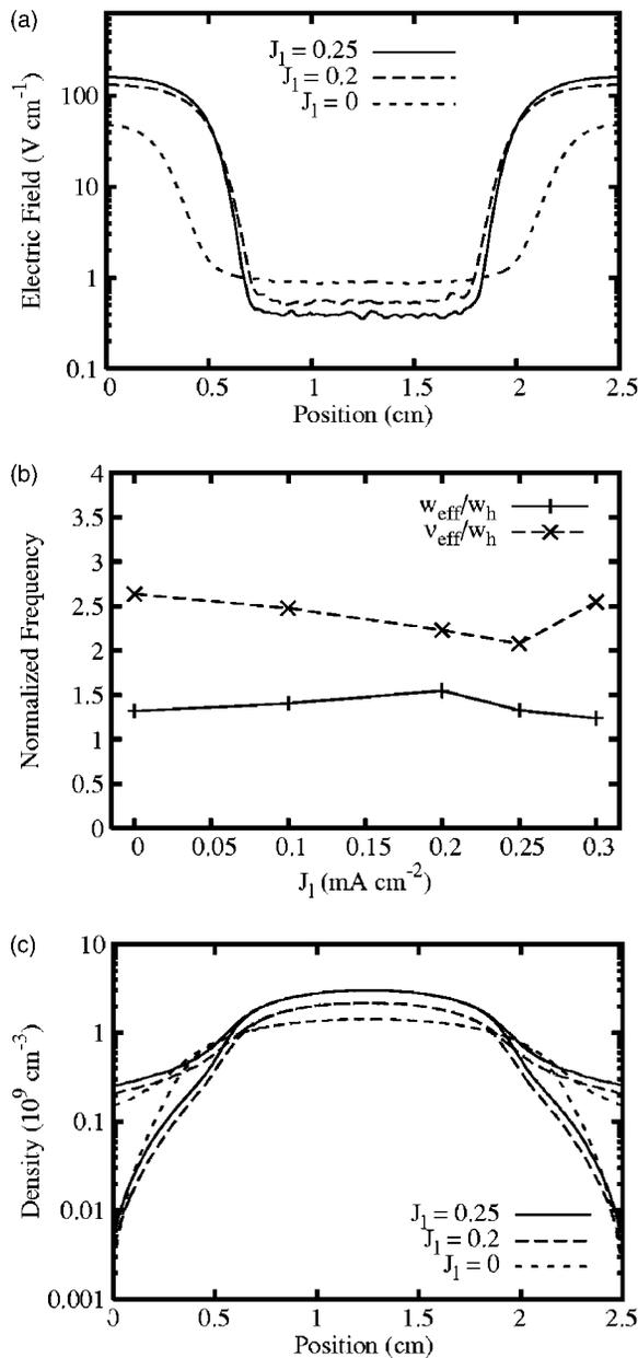
FIG. 13. Simulation result with SEE in the absence of the Ramsauer minimum: (a) The spatial profiles of the rms rf electric field. (b) Effective frequencies calculated at the discharge center. (c) The spatial profiles of the ion and electron densities.
