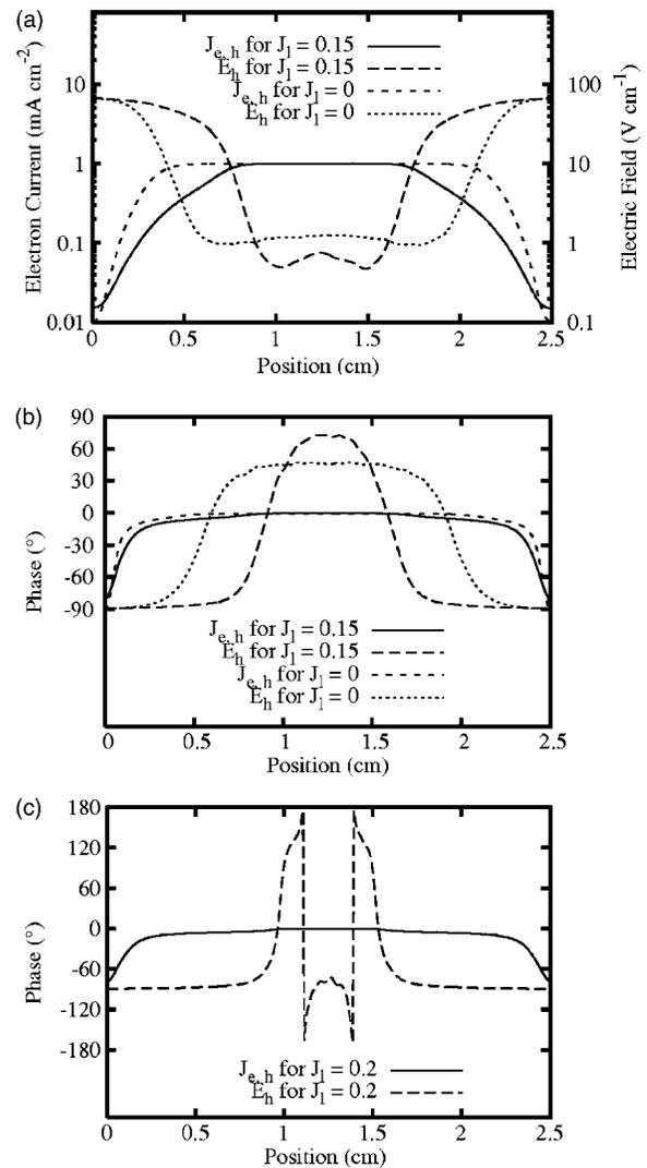
FIG. 4. Simulation result without SEE: (a) The amplitude and (b) phase of the high-frequency component of the electron current density and electric field for low-frequency currents of 0 and 0.15 mA cm<sup>-2</sup>. (c) The phase of the high-frequency component of the electron current density and electric field for the low-frequency current of 0.2 mA cm<sup>-2</sup>.
