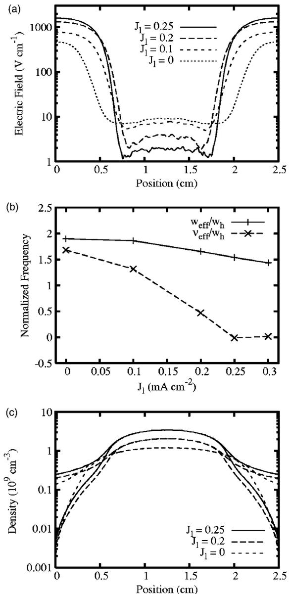
FIG. 10. Simulation result with SEE: (a) The spatial profiles of the rms rf electric field for different low-frequency currents. (b) Effective frequencies calculated at the discharge center. (c) The spatial profiles of the ion and electron densities for low-frequency currents of 0, 0.2, and 0.25 mA cm<sup>-2</sup>.
