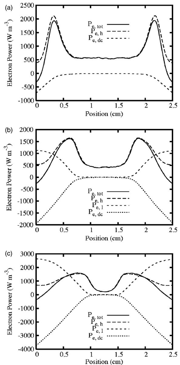
FIG. 8. Simulation result without SEE in the absence of the Ramsauer minimum: The spatial profile of the power consumed by electrons for low-frequency currents of (a) 0, (b) 0.15, and (c) 0.25 mA cm<sup>-2</sup>.
