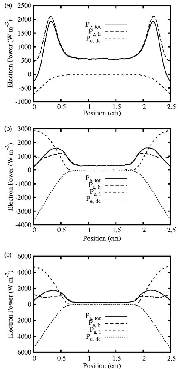
FIG. 14. Simulation result with SEE in the absence of the Ramsauer minimum. The spatial profile of the power consumed by electrons for low-frequency currents of (a) 0, (b) 0.2, and (c) 0.25 mA cm<sup>-2</sup>.
