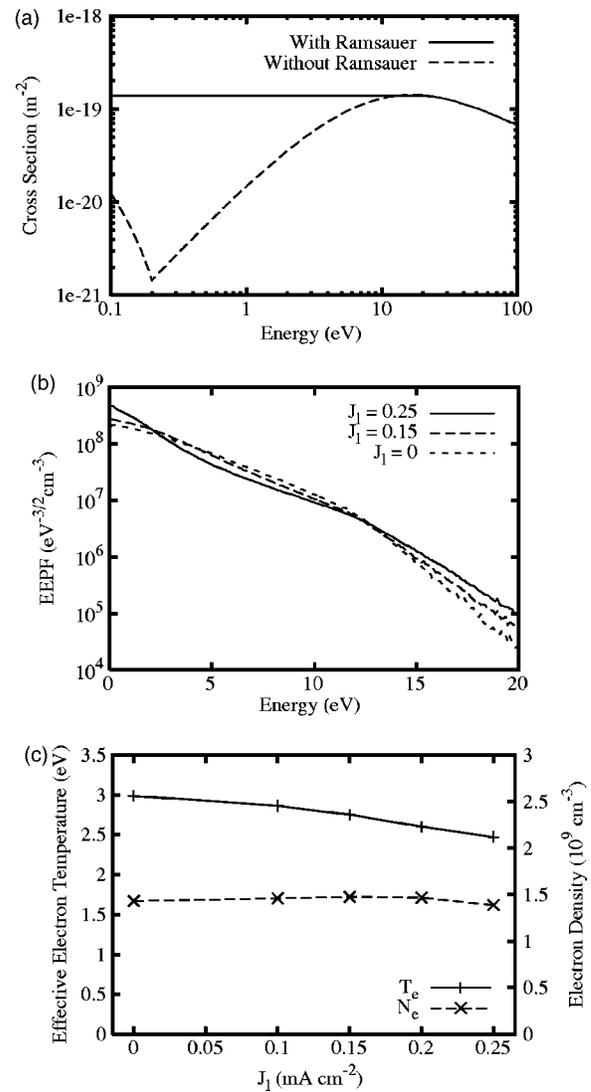
FIG. 6. Simulation result without SEE in the absence of the Ramsauer minimum: (a) Model elastic collision cross section. (b) Electron energy probability functions at the discharge center. (c) The electron temperature and electron density at the discharge center.
