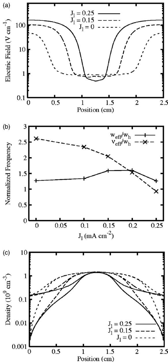
FIG. 7. Simulation result without SEE in the absence of the Ramsauer minimum: (a) The spatial profiles of the rms rf electric field. (b) Effective frequencies at the discharge center. (c) The spatial profiles of the ion and electron densities.
