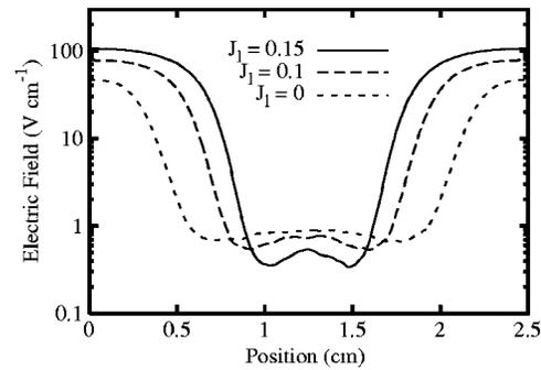
FIG. 2. Simulation result without SEE. The spatial profiles of the rms rf electric field for different low-frequency currents.
