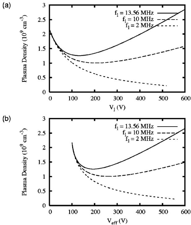
FIG. 6. Plasma densities as a function of (a) the low-frequency voltage and (b) the effective voltage for various lower frequencies with the fixed high-frequency (27 MHz) voltage ( $V_h = 100 \text{ V}$ ).
