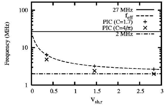
FIG. 2. Effective frequency transition for ion bombardment energy distribution functions of Fig. 1.
