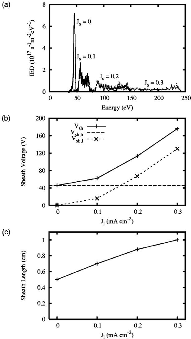
FIG. 1. PIC/MC simulation results by varying the low-frequency (2 MHz) current for the fixed high-frequency (27 MHz) current ( $J_h=2 \text{ mA cm}^{-2}$ ): (a) Ion bombardment energy distribution functions for various low-frequency current, (b) sheath voltages as a function of the low-frequency current, and (c) sheath length as a function of the low-frequency current.
