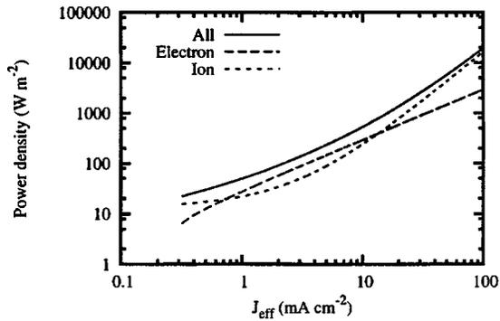
FIG. 4. Powers absorbed by electrons, ions, and all species as a function of effective current. They were obtained by varying the high-frequency (27 MHz) current for the fixed low-frequency (2 MHz) current ( $J_l = 0.22 \text{ mA cm}^{-2}$ ).
