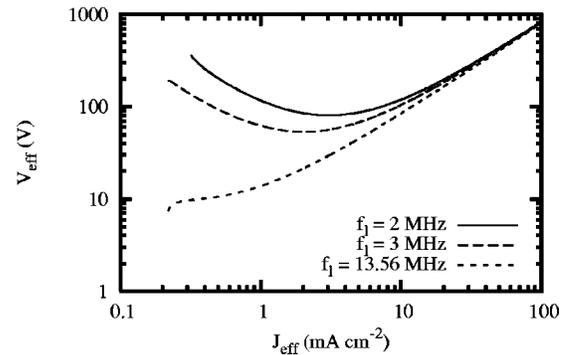
FIG. 5. Effective voltages as a function of effective current. They were obtained by varying the high-frequency (27 MHz) current for various lower frequencies with the fixed low-frequency current ( $J_l = 0.22 \text{ mA cm}^{-2}$ ).
