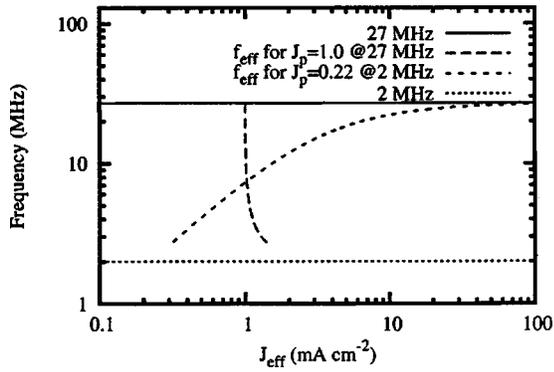
FIG. 3. Effective frequency transition for rf discharge parameters in dual rf discharges when the current of 2 or 27 MHz source varies for the fixed current of 27 or 2 MHz source to 1.0 or 0.22 mA/cm<sup>2</sup>, respectively.
