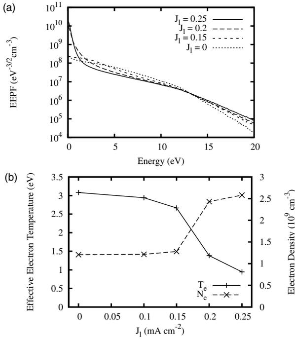
FIG. 1. Simulation result for the mode transition without SEE: (a) Electron energy probability functions at the discharge center for various low-frequency currents. (b) Effective electron temperature and electron density at the discharge center as a function of the low-frequency current. Time-averaged values were presented.
