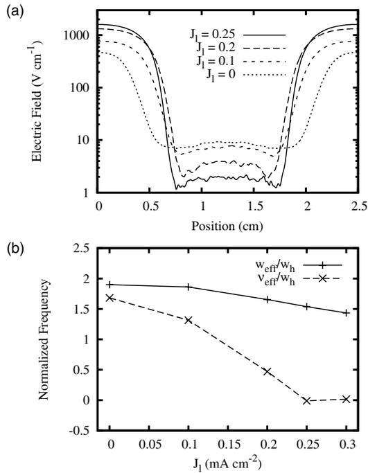
FIG. 4. Simulation result with SEE: (a) The time-averaged spatial profiles of the rf electric field for different low-frequency currents. (b) Frequencies calculated at the discharge center.
