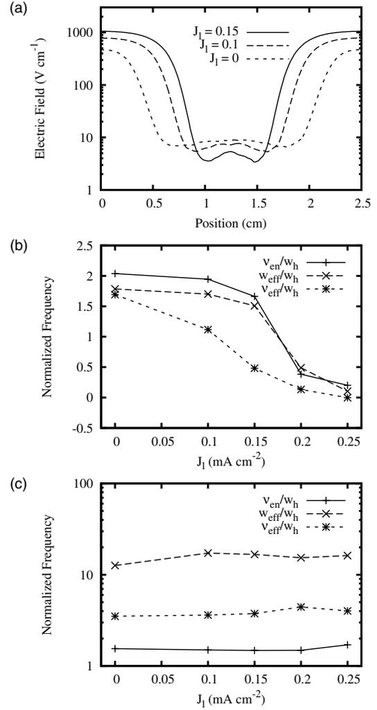
FIG. 2. Simulation result without SEE: (a) The time-averaged spatial profiles of the rf electric field for different low-frequency currents. Frequencies calculated at (b) the discharge center and (c) the position where the consumed power by electrons has the maximum value.
