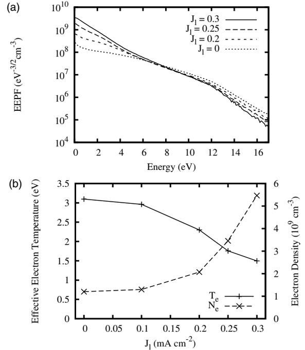
FIG. 3. Simulation result for the mode transition with SEE: (a) Electron energy probability functions at the discharge center for various low-frequency currents. (b) Effective electron temperature and electron density at the discharge center as a function of the low-frequency current.
