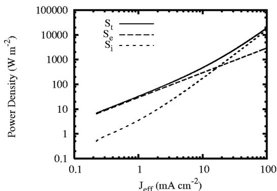
FIG. 7. The dissipated powers as a function of the effective current for the low frequency of 13.56 MHz when the high-frequency (27 MHz) current varies for the fixed low-frequency current ( $J_1 = 0.22 \text{ mA cm}^{-2}$ ).
