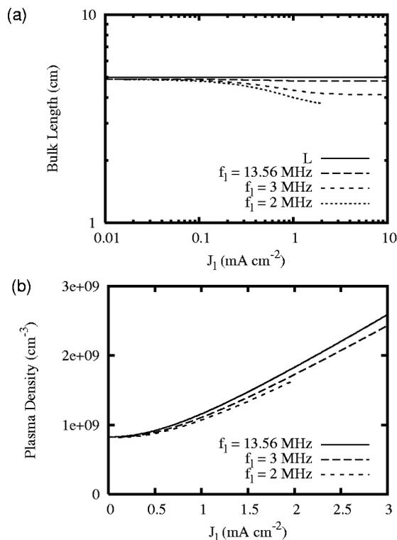
FIG. 6. For the gap distance of 5 cm, (a) the bulk plasma length and (b) the plasma density as a function of the low-frequency current ( $J_1 = 1 \text{ mA cm}^{-2}$ ).
