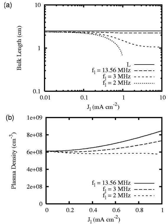
FIG. 5. For various low frequencies, (a) the bulk plasma length and (b) the plasma density as a function of the low-frequency current ( $L=2.5$  cm and  $J_h=1$  mA cm<sup>-2</sup>).
