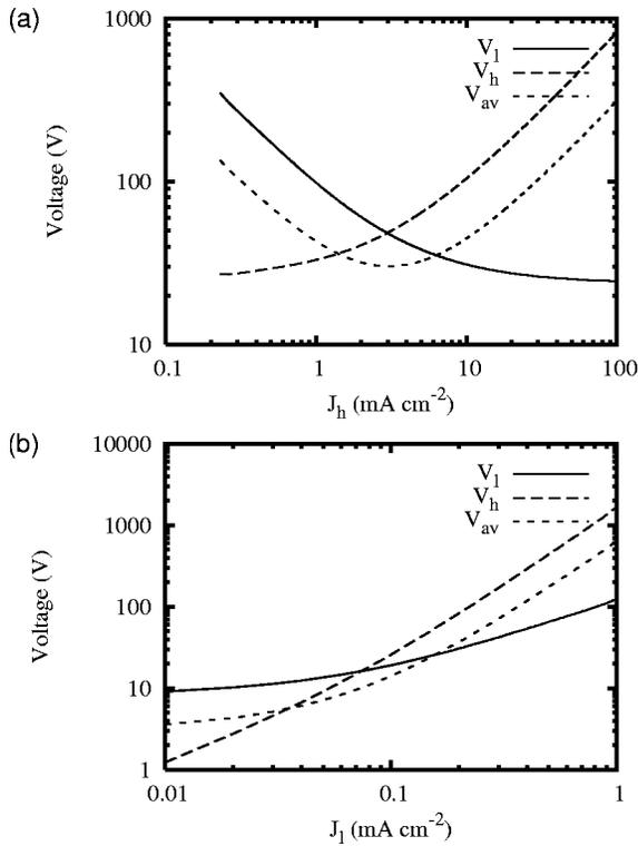
FIG. 4. The time-averaged plasma potential and the amplitudes of the low-frequency (2 MHz) and high-frequency (27 MHz) voltages as a function of (a) the high-frequency (27 MHz) current ( $J_h=0.22$  mA cm<sup>-2</sup>) and (b) low-frequency (2 MHz) current ( $J_l=1$  mA cm<sup>-2</sup>).  $V_{av}$  is the time-averaged plasma potential.
