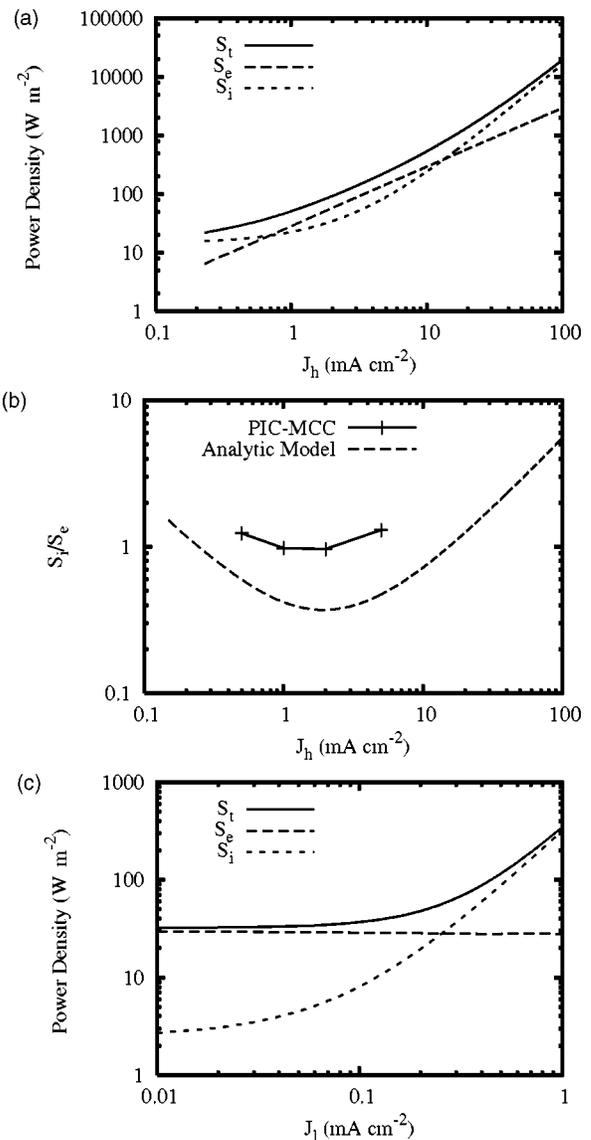
FIG. 3. Powers absorbed by electrons ions, and all species as a function of (a) the high-frequency (27 MHz) current ( $J_l=0.22 \text{ mA cm}^{-2}$ ) and (c) the low-frequency (2 MHz) current ( $J_h = 1 \text{ mA cm}^{-2}$ ). (b) The ratio of the ion to electron power as a function of the high-frequency (27 MHz) current ( $J_l=0.14 \text{ mA cm}^{-2}$ ).
