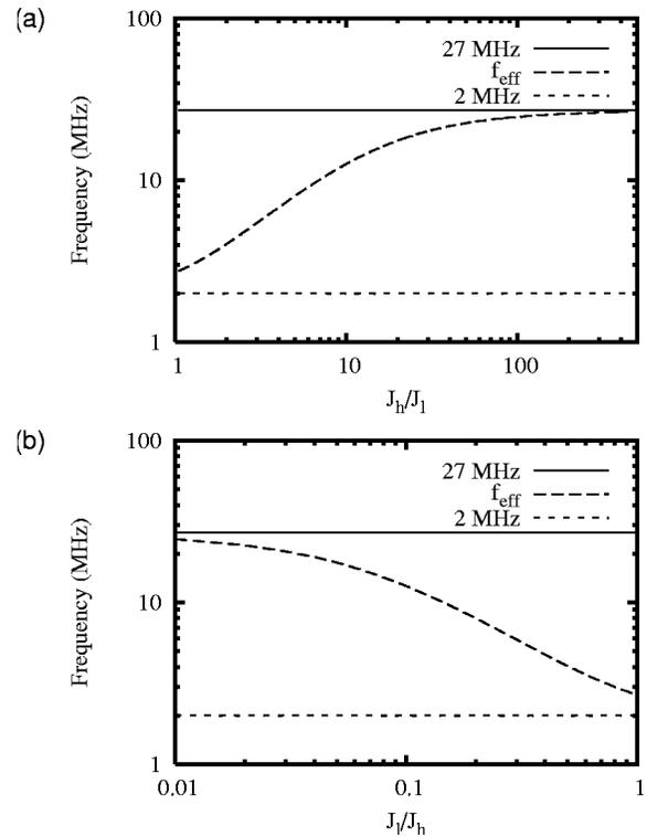
FIG. 1. Effective frequency transitions (a) when the high-frequency (27 MHz) current increases for the fixed low-frequency (2 MHz) current ( $J_l = 0.22$  mA cm<sup>-2</sup>) and (b) when the low-frequency (2 MHz) current varies for the fixed high-frequency (27 MHz) current ( $J_h = 1$  mA cm<sup>-2</sup>).
