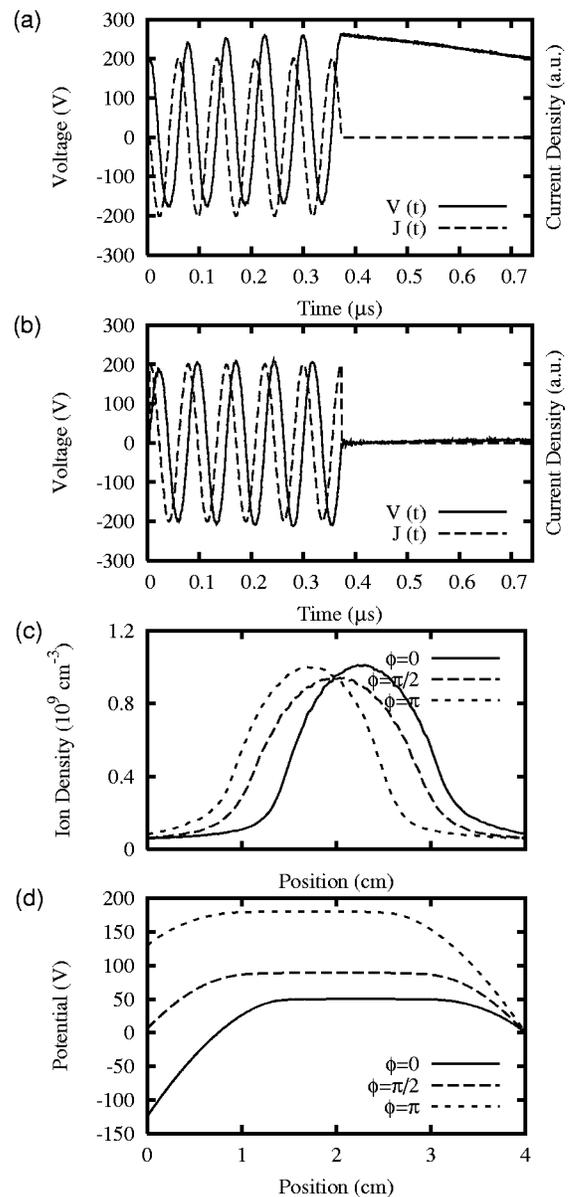
FIG. 2. The time evolutions of the voltage and current on the powered electrode for the rf phases of (a)  $\pi$  and (b)  $\pi/2$ . The spatial profiles of (c) the ion density and (d) potential for various rf phases.
