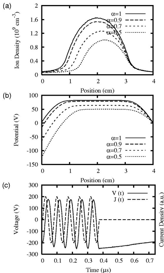
FIG. 1. The spatial profiles of (a) the ion density and (b) potential for various duty ratios. (c) The time evolutions of the voltage and current on the powered electrode for the duty ratio of 0.5.
