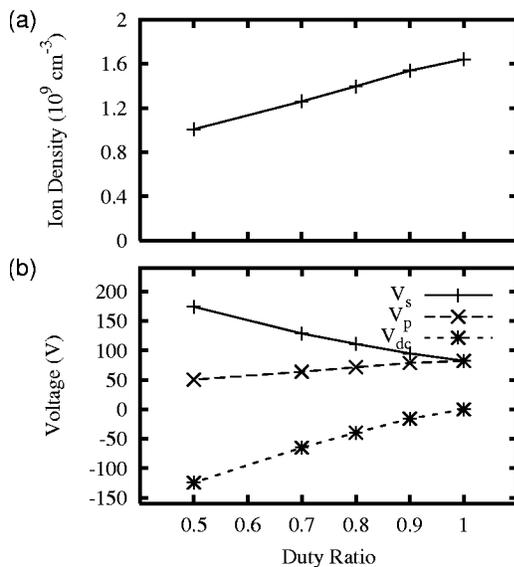
FIG. 3. (a) The ion peak density and (b) voltages as a function of the duty ratio.  $V_p$ ,  $V_{dc}$ , and  $V_s$  represent the plasma potential, dc bias, and the time-averaged sheath voltage, respectively.
