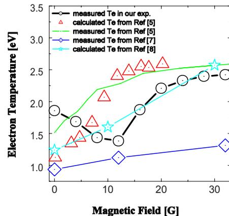
FIG. 1. (Color online) The evolution of electron temperatures ( $T_{\text{eff}}$ ) with magnetic field at a low pressure capacitive discharge (circle: measured  $T_{\text{eff}}$  in our experiment, triangle: calculated  $T_{\text{eff}}$  in Ref. 5, dot: measured  $T_{\text{eff}}$  in Ref. 5, diamond: measured  $T_{\text{eff}}$  in Ref. 7, star: calculated  $T_{\text{eff}}$  in Ref. 8).
