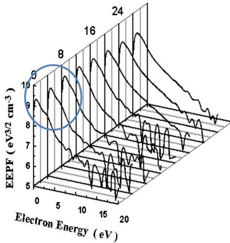
FIG. 2. (Color online) Measured EEPFs for various magnetic fields at 10 mTorr, 1 A, and 2 cm gap.
