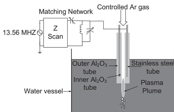
**Figure 1.** Schematic of the experimental setup and electrode configuration for creating hybrid gas/liquid plasmas.
