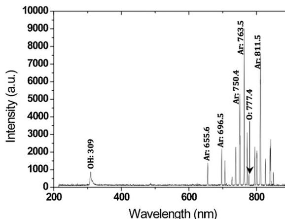
Figure 4. Typical optical emission spectrum from a glow discharge in hybrid gas/liquid plasma.
