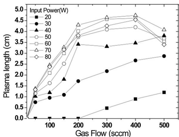
Figure 3. Plasma plume length injected into water, as measured by total optical emission as a function of argon gas flow rate.
