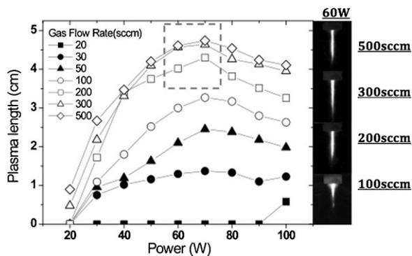
Figure 2. Plasma plume length injected into water, as measured by total optical emission as a function of the applied RF power. Each line corresponds to one gas flow rate. The red box is optimal points according to the plum length saturation. The side pictures are comparing the plume lengths measured at 60 W. The gas flow is 100, 200, 300 and 500 sccm from bottom to the top.
