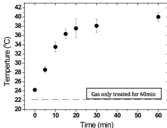
Figure 9. The temperature of plasma treated DI water versus plasma treatment time. The temperature does not exceeded  $40^\circ\text{C}$  even after 60 min of plasma treatment.
