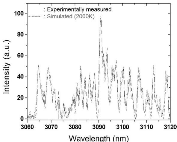
Figure 5. Comparison of both measured OH band spectra and simulated spectra (LIFbase) for the determination of the rotational temperature of hybrid plasma at 60 W RF input power.
