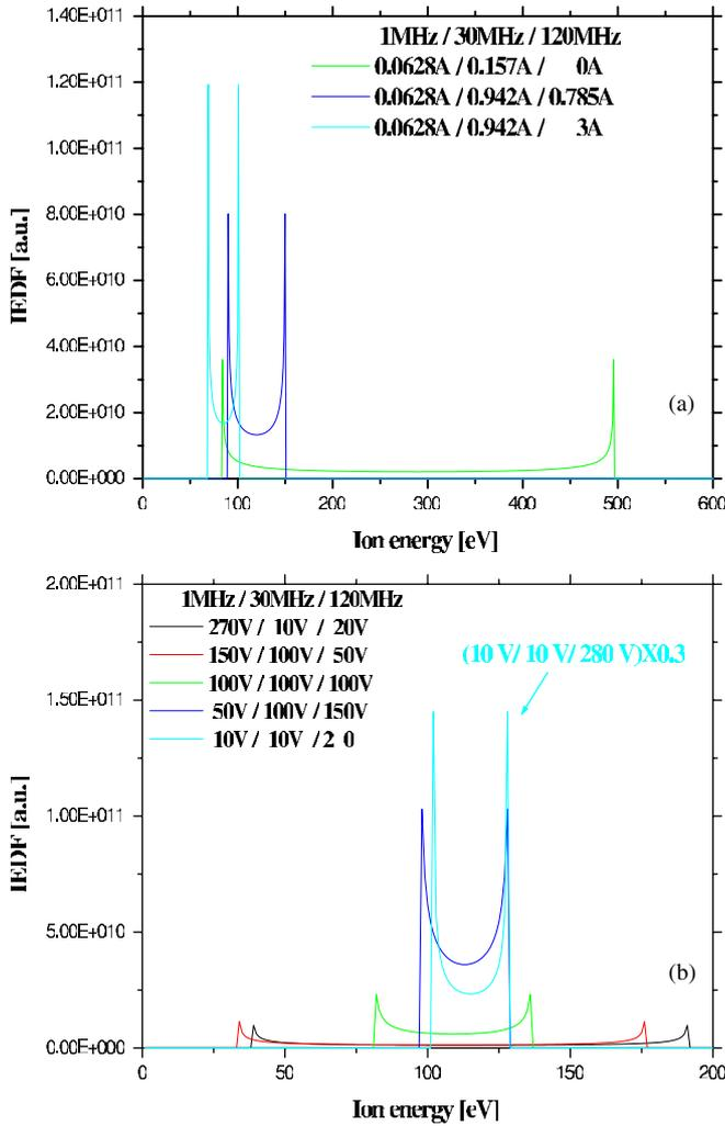
**Figure 6.** Analytical calculations of IEDFs in a collisionless rf sheath model through the effective frequency. (a) IEDFs with respect to the current ratio; (b) IEDFs with respect to the voltage ratio.
