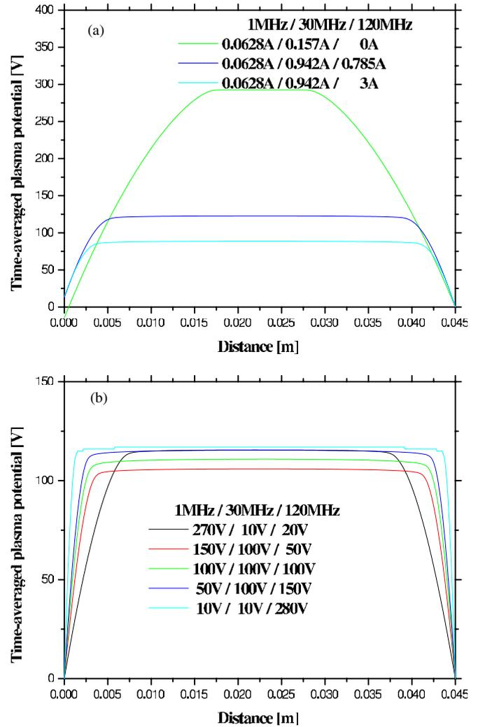
**Figure 3.** (a) Time-averaged plasma potential profile with the current ratio of the triple-frequency (1, 30 and 120 MHz) source; (b) time-averaged plasma potential profile with the voltage ratio of the triple-frequency (1, 30 and 120 MHz) source.
