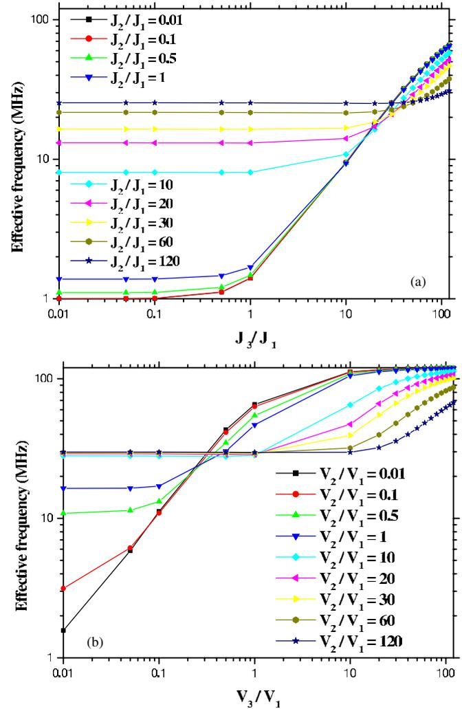
**Figure 2.** (a) Effective frequency with respect to the current density ratio of the triple-frequency source; (b) effective frequency with respect to the voltage ratio of the triple-frequency source.
