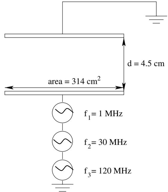
**Figure 1.** Schematic diagram of low-pressure (10 mTorr) argon plasmas sustained by the triple-frequency (1, 30 and 120 MHz) source in symmetrical current-driven and voltage-driven capacitively coupled plasma reactors.
