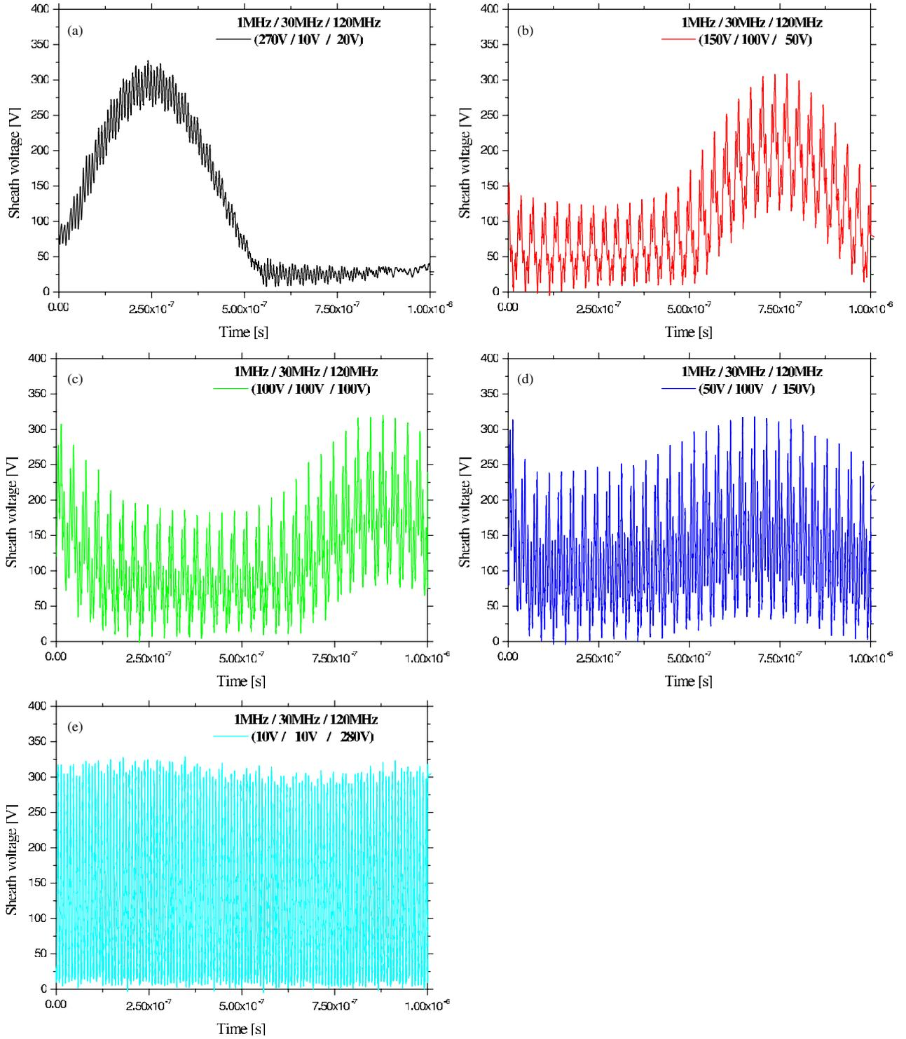
**Figure 5.** Sheath voltage profile over one period of 1 MHz calculated from the 1D PIC-MCC simulation with the voltage ratio of the triple-frequency (1, 30 and 120 MHz) source. (a) 270 V/10 V/20 V; (b) 150 V/100 V/50 V; (c) 100 V/100 V/100 V; (d) 50 V/100 V/150 V; (e) 10 V/10 V/280 V.
