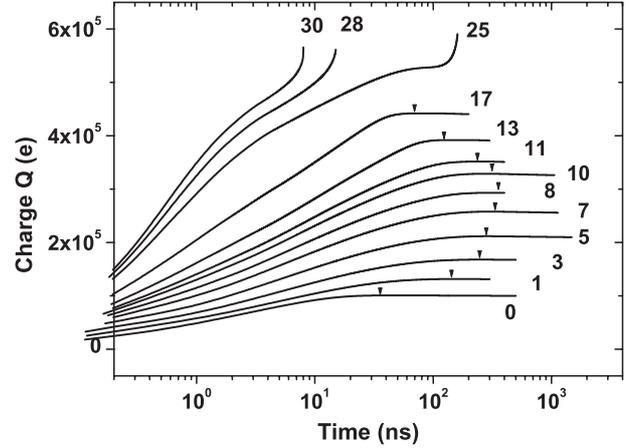
**Figure 13.** Particle charge as a function of time for the different values of  $E_{\text{ext}}$  ( $\text{kV cm}^{-1}$ ) that label the curves. The arrows indicate the moment when the grain charge attains its maximal value.
