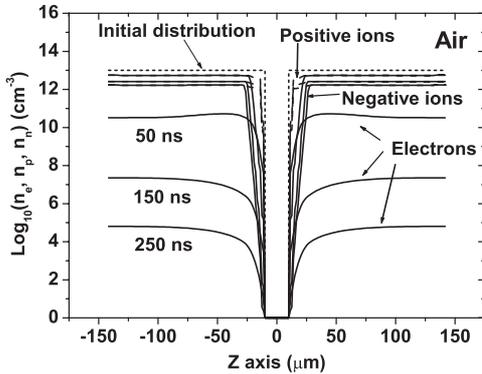
**Figure 5.** Evolution of electrons and positive and negative ions around the dust grain (along  $z$ -axis) during the first 250 ns of the dust grain charging in a decaying air plasma (zero external field). The curves are shown for three successive time moments. The centre of the dust grain is located at  $z = 0$ .
