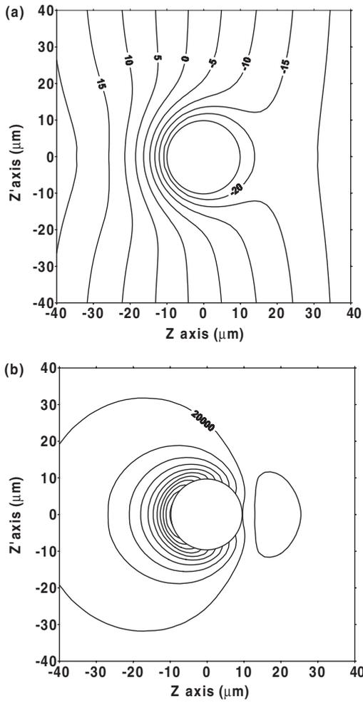
**Figure 11.** Contours of (a) potential and (b) absolute value of the electric field around the conducting dust grain after 30 ns of the charging process in the external field,  $E_{\text{ext}} = 5000 \text{ V cm}^{-1}$ . (The contour lines for the electric field are shown in  $4000 \text{ V cm}^{-1}$ .)
