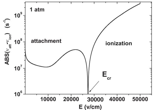
**Figure 4.** Absolute value of the difference between electron attachment and ionization rates.
