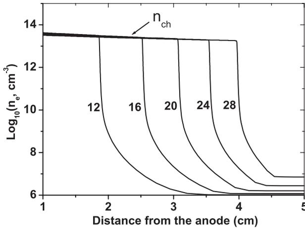
**Figure 2.** Profiles of electron number density at the streamer axis at five successive time moments. Notation is as in figure 1.
