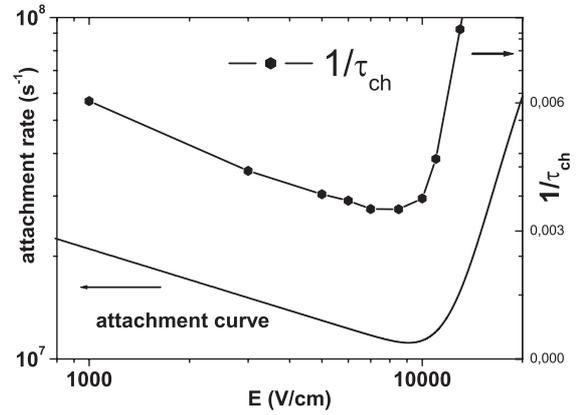
**Figure 14.** Correlation between the attachment rate curve and charging time,  $\tau_{\text{ch}}$  (time needed for the grain to attain the maximal charge).
