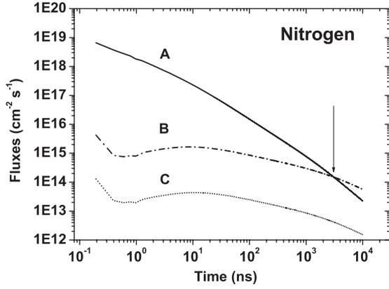
**Figure 8.** Diffusion and drift fluxes of charged particles collected by the spherical dust grain in decaying plasma (nitrogen). Curve A, diffusion flux of electrons; curve B, drift flux of positive ions; curve C, diffusion flux of positive ions.
