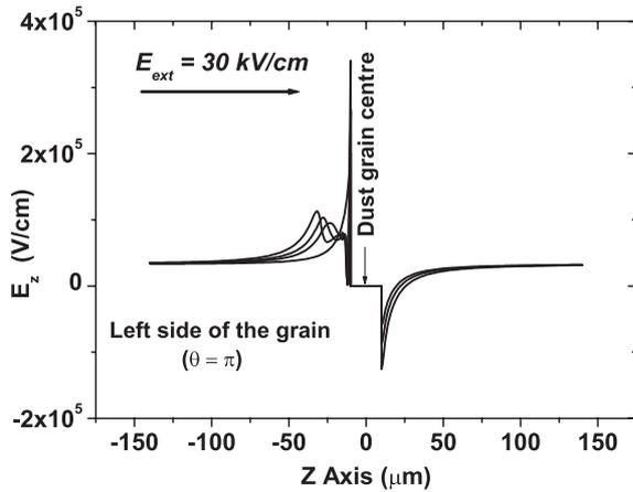
**Figure 15.** Corona discharge starting from the dust grain. Distribution of the z-component of the electric field at three successive time moments.
