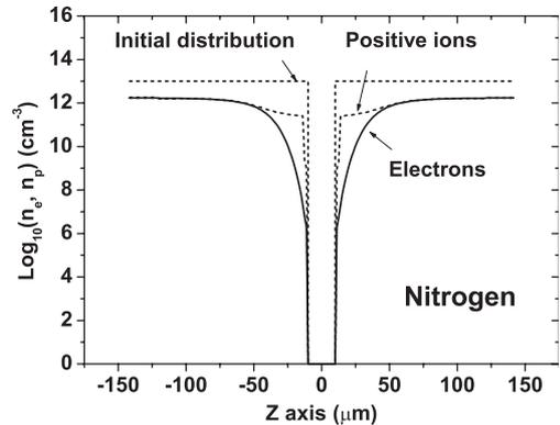
**Figure 7.** Distribution of electrons and positive ions around the dust grain in decaying nitrogen plasma at 10 000 ns (zero external field). The centre of the dust grain is located at  $z = 0$ .
