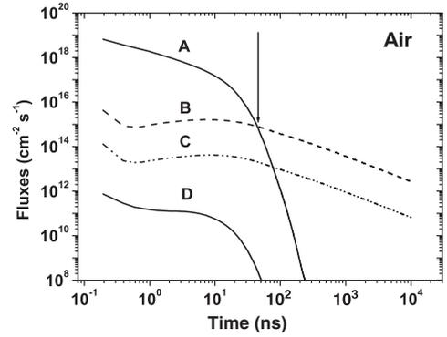
**Figure 6.** Diffusion and drift fluxes of charged plasma particles collected by the spherical dust grain in decaying plasma (air). Curve A, diffusion flux of electrons; curve B, drift flux of positive ions; curve C, diffusion flux of positive ions; and curve D, diffusion flux of negative ions.
