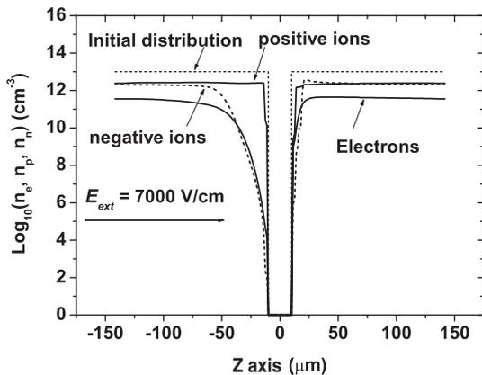
**Figure 12.** The asymmetric profile of charged particle distribution around the dust grain (along  $z$ -axis) after 250 ns charging in an external field of  $7000 \text{ V cm}^{-1}$ . The direction of the external field is indicated by the arrow.
