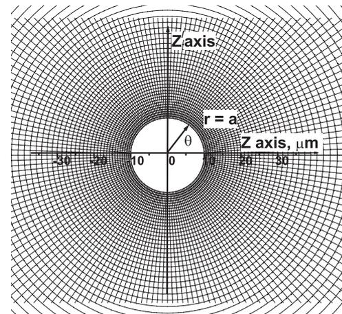
**Figure 3.** Spherical axisymmetrical mesh.
