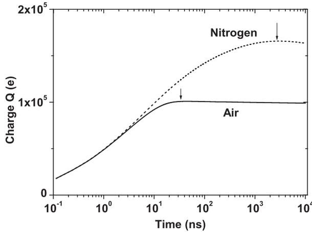
**Figure 9.** Time evolution of charge accumulated on the dust grain in decaying air and nitrogen plasmas in zero external field. The arrows indicate the moment when the charge attains its maximal value.
