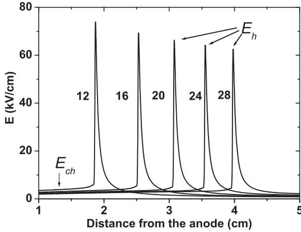
**Figure 1.** Positive (cathode-directed) streamer development in atmospheric air in a sphere–plane gap (the sphere radius is 0.05 cm and the applied voltage is 5 kV). Profiles of absolute value of the electric field at the streamer axis at five successive time moments are presented. Numbers near the lines denote the time in nanoseconds.
