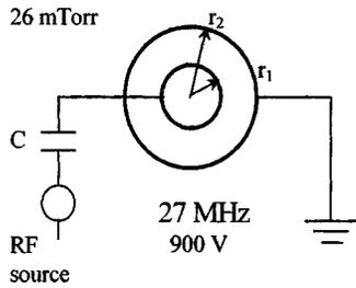
FIG. 1. Schematic diagram of cylindrical capacitively coupled plasma source.
