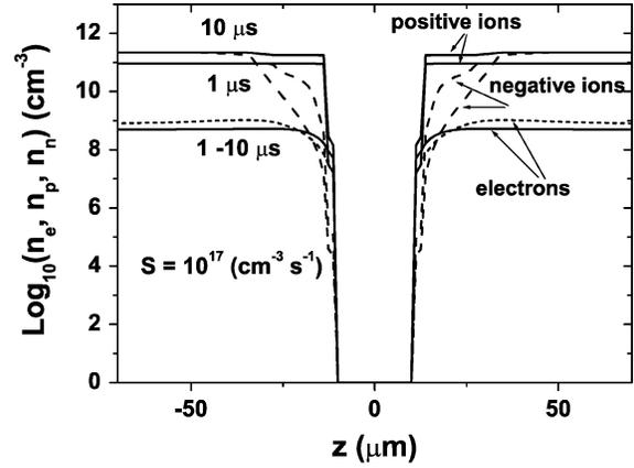
Fig. 3. Strong external source  $S = 10^{17} \text{ cm}^{-3} \text{ s}^{-1}$ . Distribution of electrons and ions around the dust grain in developing plasma for two time moments  $1 \mu\text{s}$  and  $10 \mu\text{s}$ . The center of the dust grain is located at  $z = 0$ . The background electron concentration arrives to the steady state very quickly.
