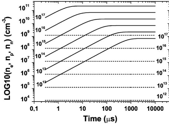
Fig. 2. Evolution of electron (dashed lines) and ion (solid lines) concentration in the bulk plasma for different values of external source intensity. Numbers at the lines denote the source intensity ( $\text{cm}^{-3} \text{s}^{-1}$ ). Initial concentrations at  $t = 0$  are  $n_e = n_p = 10^3 \text{ cm}^{-3}$ . Calculation according to (11) and (14) with  $\beta_{ii} = 2 \times 10^{-6} \text{ cm}^3 \text{ s}^{-1}$ ,  $\nu_{\text{att}} = 8 \times 10^7 \text{ s}^{-1}$ .
