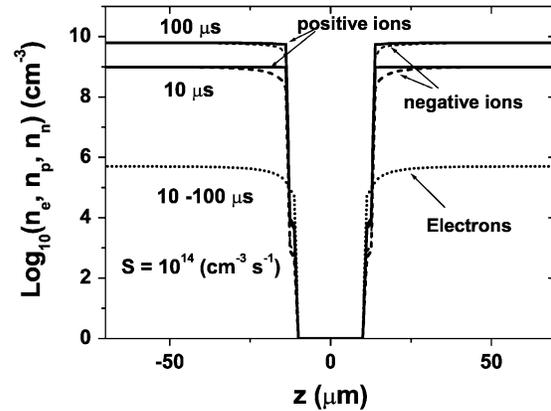
Fig. 6. Weak external source  $S = 10^{14} \text{ cm}^{-3} \text{ s}^{-1}$ . Distribution of electrons and ions around the dust grain in developing plasma for two time moments 10 and 100  $\mu\text{s}$ . The center of the dust grain is located at  $z = 0$ .
