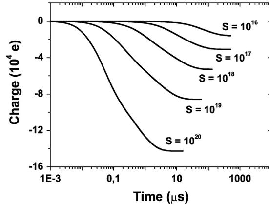
Fig. 5. Time evolution of charge accumulated on the dust grain in developing air plasma for different values of strong external source  $S$ .
