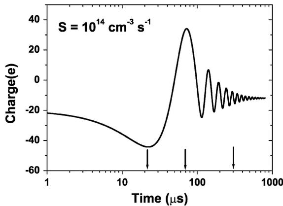
Fig. 8. Time evolution of charge accumulated on the dust grain in developing air plasma for weak external source  $S = 10^{14} \text{ cm}^{-3} \text{ s}^{-1}$ . Oscillating regime of the dust-grain charge is demonstrated.
