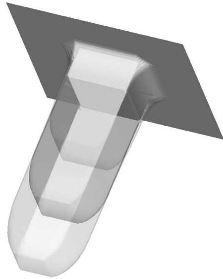
Fig. 5. The Lax–Friedrichs scheme ( $R_x = 1$ ,  $R_y = 1$ ,  $R_z = 1$ ): The etching profiles for  $V = V_0 \cos \theta$  at  $t = 0$ ,  $t = 20$  s,  $t = 40$  s and  $t = 60$  s.
