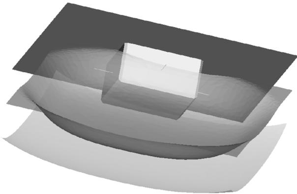
Fig. 4. The Lax–Friedrichs scheme ( $R_x = 1$ ,  $R_y = 1$ ,  $R_z = 1$ ): The etching profiles for  $V = V_0(1 + 4 \sin^2 \theta) \cos \theta$  at  $t = 0$ ,  $t = 9$  s and  $t = 15$  s.
