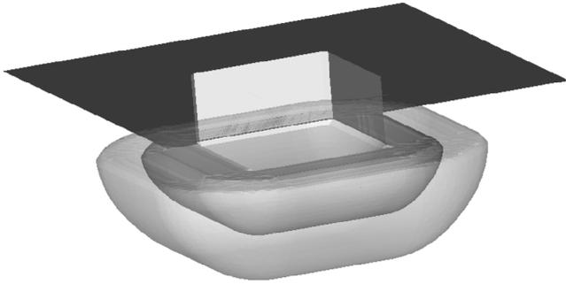
Fig. 3. The upwind scheme: The etching profiles for  $V = V_0$  at  $t = 0$ ,  $t = 9$  s and  $t = 15$  s.
