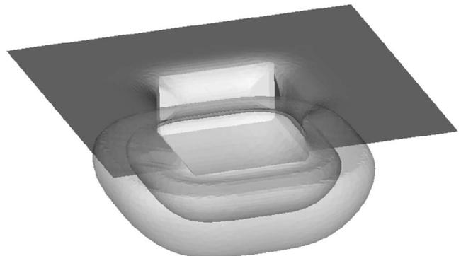
Fig. 2. The Lax–Friedrichs scheme ( $R_x = 1$ ,  $R_y = 1$ ,  $R_z = 1$ ): The etching profiles for  $V = V_0$  at  $t = 0$ ,  $t = 9$  s and  $t = 15$  s.
