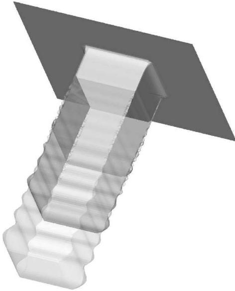
Fig. 7. The Lax–Friedrichs scheme ( $R_x = 1$ ,  $R_y = 1$ ,  $R_z = 0.1$ ): The etching profiles for  $V = V_0 \cos \theta$  at  $t = 0$ ,  $t = 20$  s,  $t = 40$  s and  $t = 60$  s.
