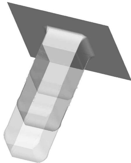
Fig. 6. The Lax–Friedrichs scheme ( $R_x = 1$ ,  $R_y = 1$ ,  $R_z = 0.3$ ): The etching profiles for  $V = V_0 \cos \theta$  at  $t = 0$ ,  $t = 20$  s,  $t = 40$  s and  $t = 60$  s.
