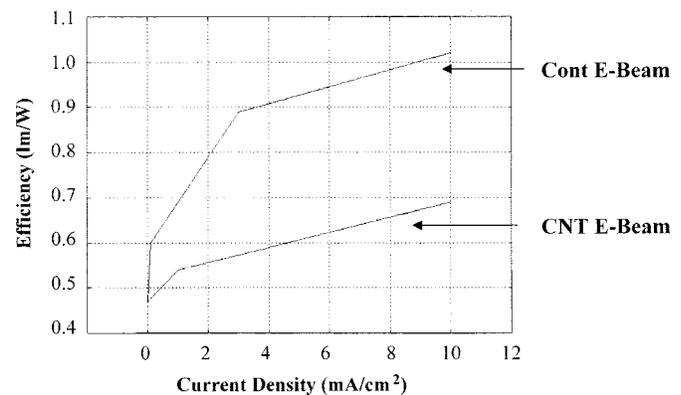
Fig. 7. Luminous efficiency comparison for the CNT E-beam and Continuous E-beam cases, at various beam current densities. The efficiency of the latter is considerably larger than the former.
