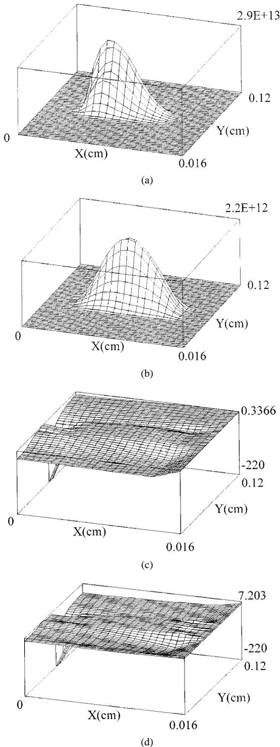
Fig. 8. Electron density distributions for no-beam, and beam cases are shown in (a) and (b), respectively. Similarly, (c) and (d) represent the potential distributions for the no-beam and beam cases respectively.
