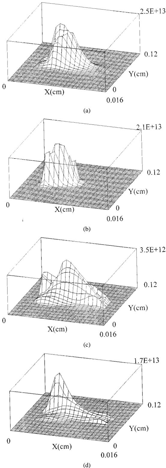
Fig. 4. (a) and (b) show ionized and excited Xe ( $Xe^*(3P_1)$ ) density distribution when the beam is off. Notice that  $Xe^+$  density is larger than  $Xe^*$  density. (c) and (d) show ionized and excited Xe density distribution when the beam is on.  $Xe^*$  density is larger than  $Xe^+$  density.
