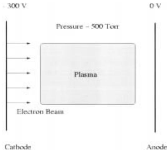
Fig. 1. Schematic of typical 1-D capacitively gas discharge model. Cathode on the left is maintained at  $-300$  V, anode is at  $0$  V. Electron beam is injected through the cathode. Beam current density and pressure are  $10$  mA/cm<sup>2</sup> and  $500$  torr, respectively.
