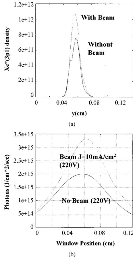
Fig. 5. (a)  $Xe^*$  density distribution near the phosphor dielectric. Upper curve stands for the beam case, while the lower curve corresponds to the no-beam case. (b) Light distribution for the beam and no-beam cases, when the sustained voltage is 220 V.
