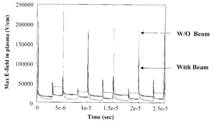
Fig. 9. Space-averaged maximum profile of electric field at different time intervals is shown. Thin lines represent the electric field when beam component is absent. Thick lines correspond to electric field when the beam component is present. The effect of beam is to reduce the electric field in the plasma.
