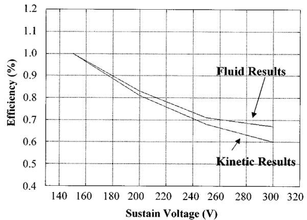
Fig. 2. A comparison of the normalized efficiency trend obtained from 1-D fluid (upper curve) and kinetic (lower curve) codes. The two results show qualitatively similar characteristics and, hence, validate the fluid treatment.
