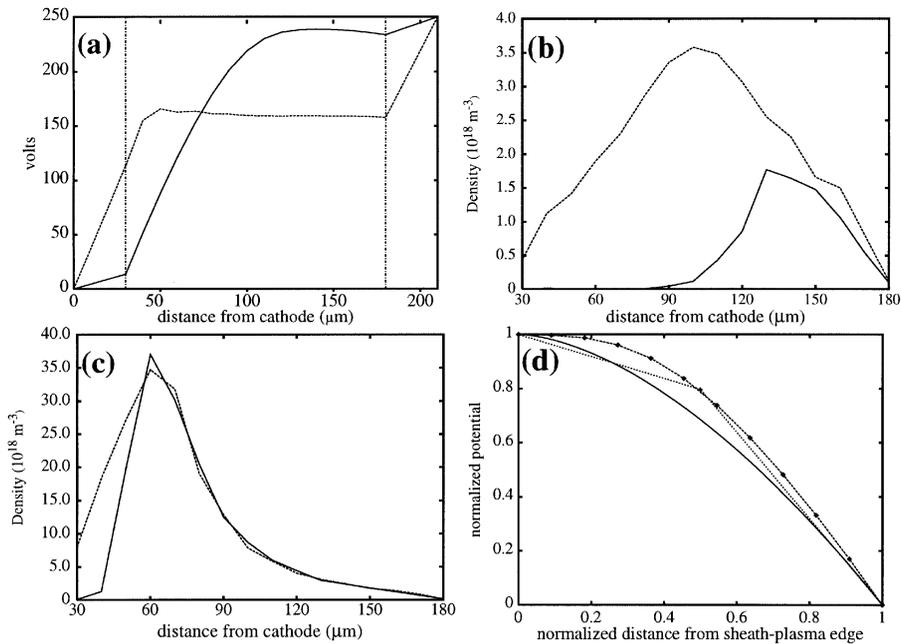
Fig. 3. Kinetic simulations, the cross section along the  $y$ -direction at the center of  $V_x$  electrode: (a) potential profile at 22 ns (solid), 37 ns (dotted) dielectric layer (solid and dotted), (b) and (c) electron (solid) and ion (dotted) density cross section at the center of the electrode at 22 ns and 37 ns, (d) the normalized potential profile, comparison of the results obtained from theory (solid) with those from the simulation (dots for 22 ns and dotted line for 37 ns).
