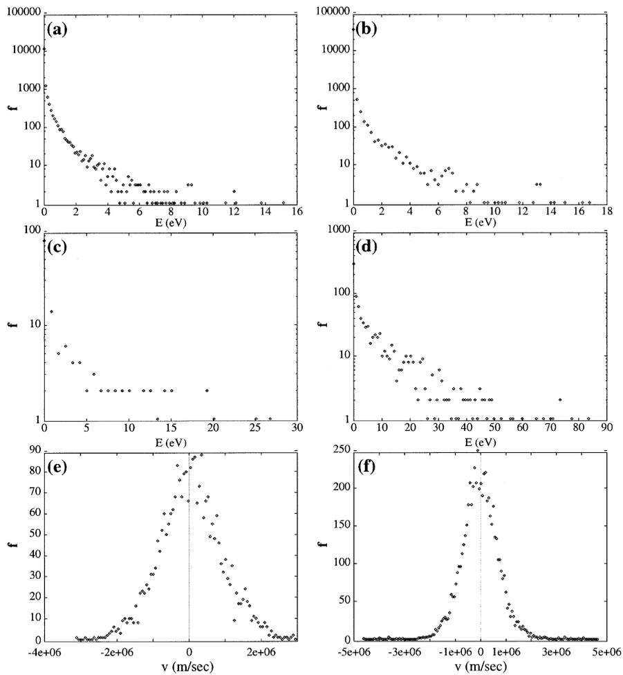
Fig. 2. Kinetic energy distributions: (a) and (b) for the ion energy distribution in the bulk plasma at 22 ns (100–180  $\mu\text{m}$ ) and 37 ns (55–180  $\mu\text{m}$ ), (c) and (d) for the ion energy distribution of the cathode sheath at 22 ns (30–35  $\mu\text{m}$ ) and 37 ns (30–35  $\mu\text{m}$ ), (e) and (f) for the electron velocity distribution in bulk plasma at 22 ns and in the cathode sheath at 37 ns.
