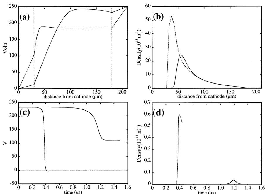
Fig. 4. Fluid simulation, the cross section along the  $y$ -direction at the center of  $V_x$  electrode: (a) potential, (b) electron and ion density, (c) potential difference between dielectric layers, (d) average electron density with  $\gamma_{\text{Neon}} = 0.5$  (dotted) and 0.05 (solid).
