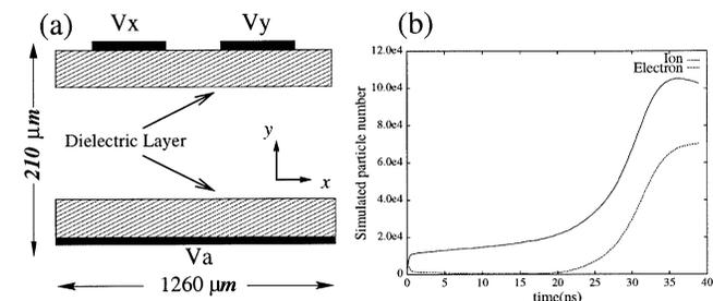
Fig. 1. (a) Cell geometry,  $1260 \times 210 \mu\text{m}^2$ ,  $V_x = 250 \text{ V}$ ,  $V_y = V_a = 0 \text{ V}$ , dielectric constant  $\epsilon_r = 10$ . (b) Kinetic simulation of number of ions (solid) and electrons (dashed), each particle represents the density  $1.890 \times 10^{15} \text{m}^{-3}$ .
